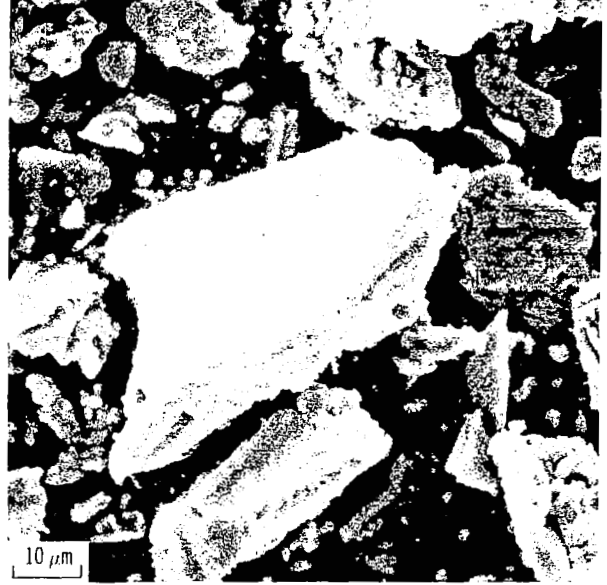
(e) Layered particle showing rub surface distress.
