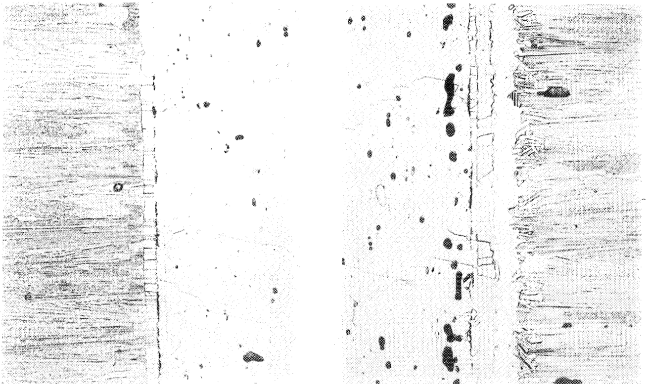
(b-2) (\gamma/\gamma' - \delta) /NiCrAl interface. X250.
