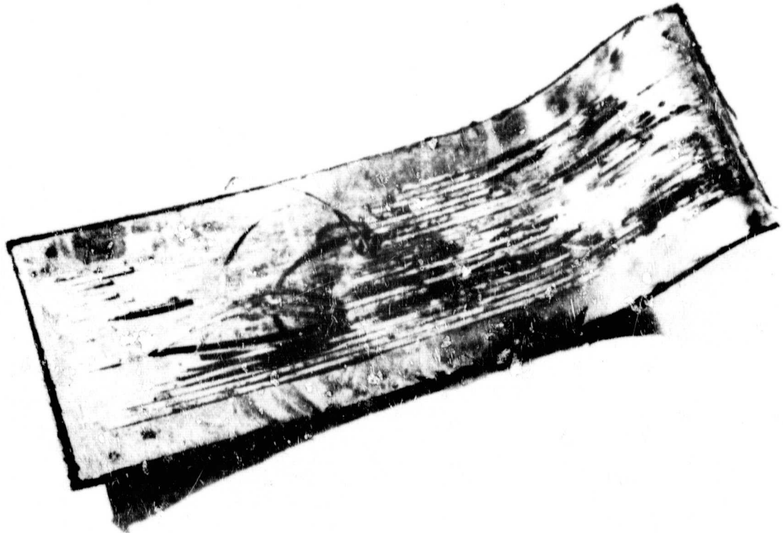
Figure 6. Electroformed Nickel Cover After Separation From NASA Test Part Showing Aluminum Strips Which Were Not Dissolved
