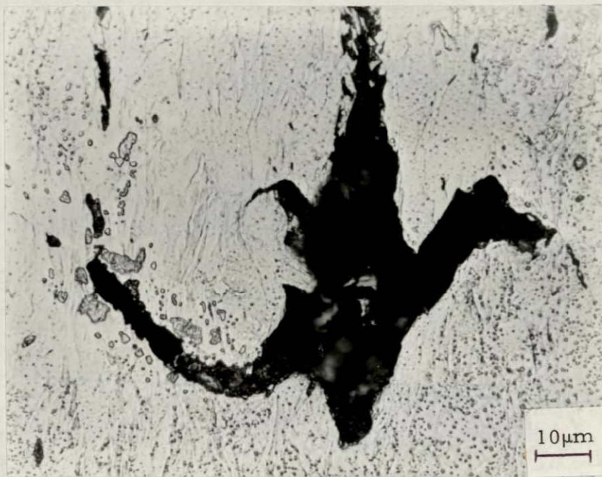
Figure 19 Optical micrograph of a sectioned tensile specimen of the 718 \text{ MN/m}^2 (104 ksi) material strained to 1.550. The tensile axis is vertical.
