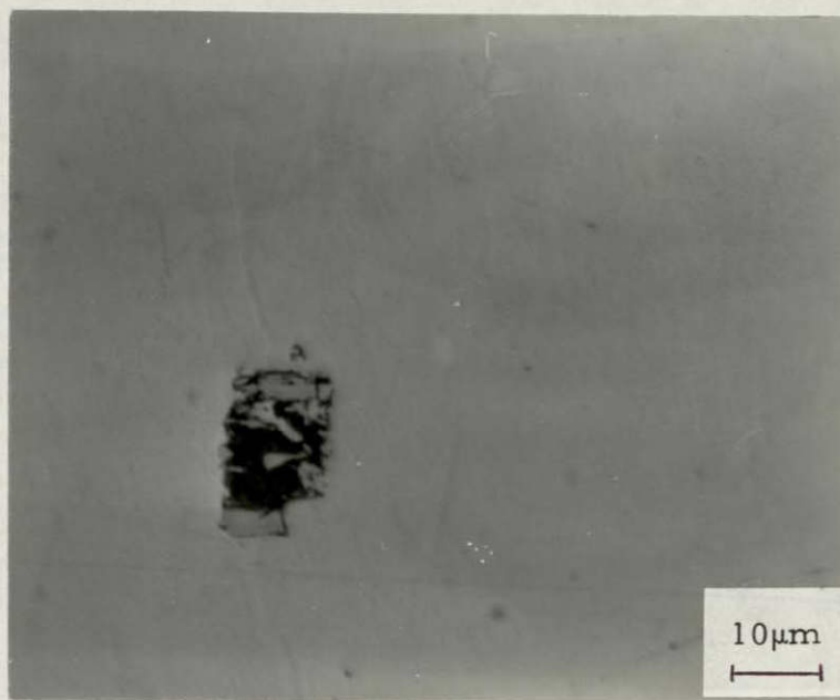
Figure 17 Optical micrograph from a sectioned tensile specimen of the 2070 \text{ MN/m}^2 (300 ksi) material strained to 0.487. Tensile axis is vertical.
