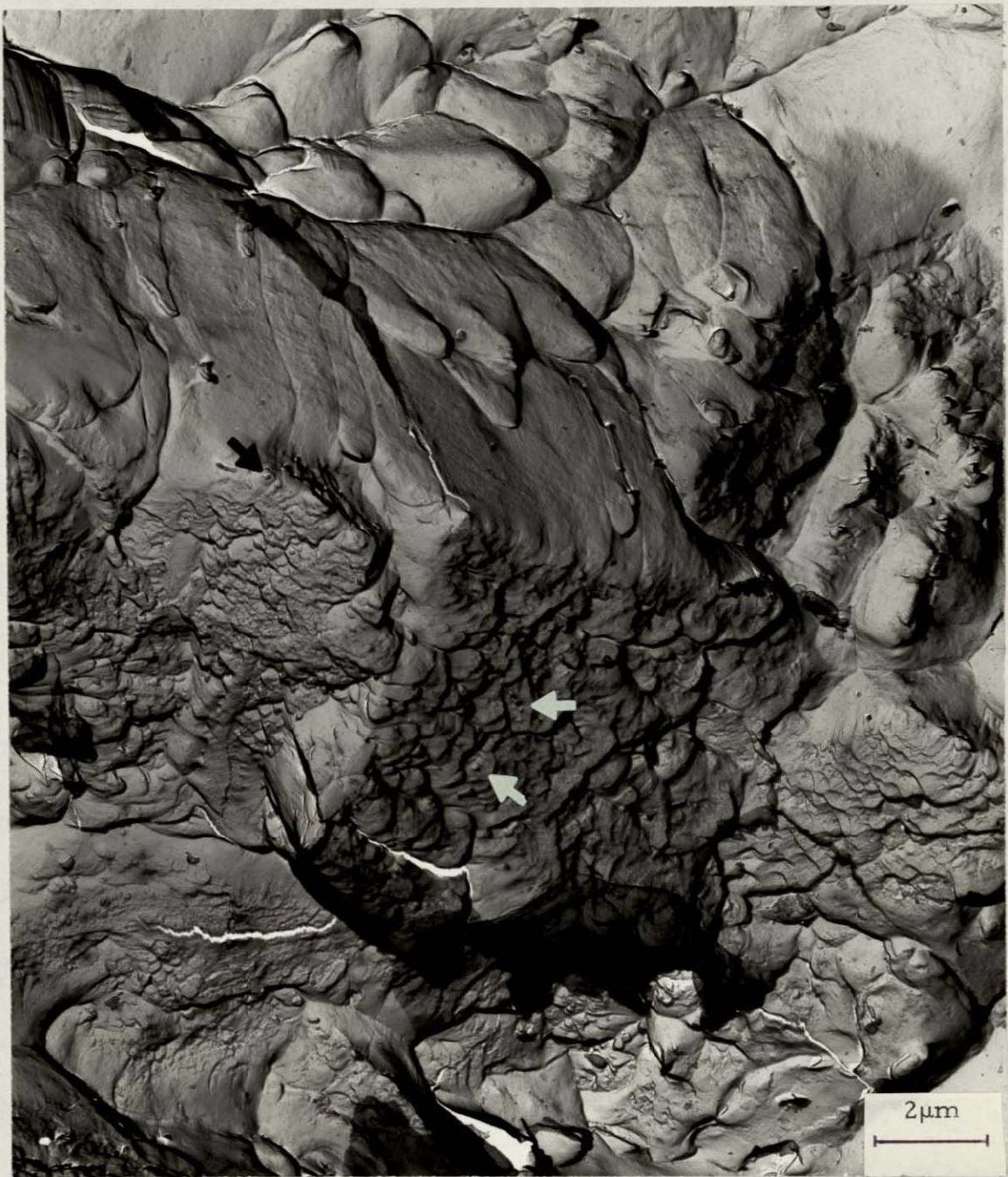
Figure 14 TEM replica fractograph from a K_{IC} fracture of the 2070 \text{ MN/m}^2 (300 ksi) yield strength condition. (Impressions of nucleation sites the size of strengthening precipitates are indicated by arrows).
