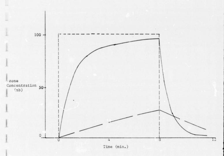
Figure 4. Response of ECC ozonesonde (2A239) with contaminated sensor cells to step changes in ozone concentration.
