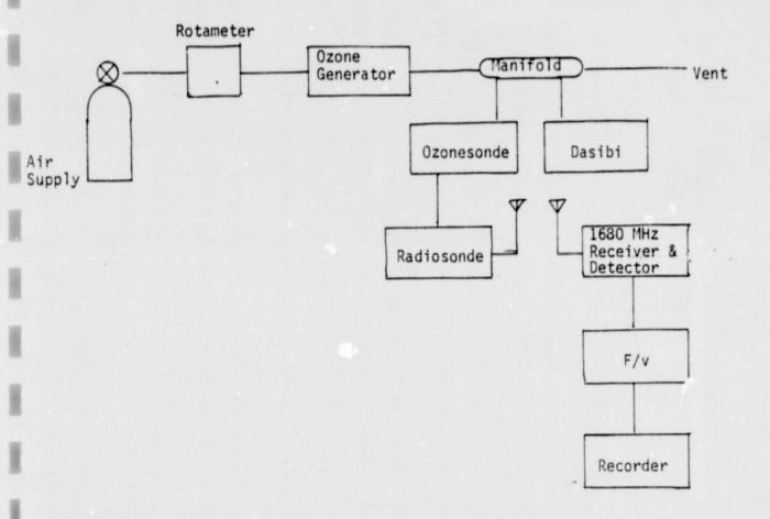
Figure 3. ECC Ozonesonde Calibration Apparatus
