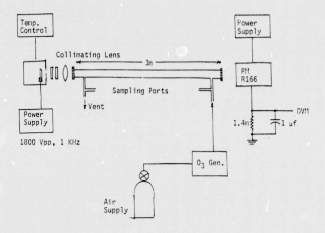
Figure 1. Ultraviolet absorption photometer for ozone calibrations.
