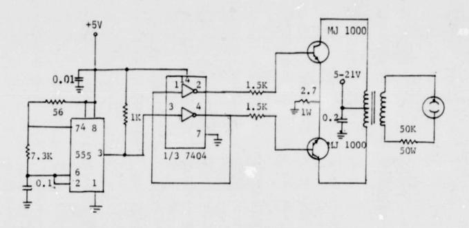
Figure 2. Partial schematic for lamp power supply for ultraviolet absorption ozone photometer.
