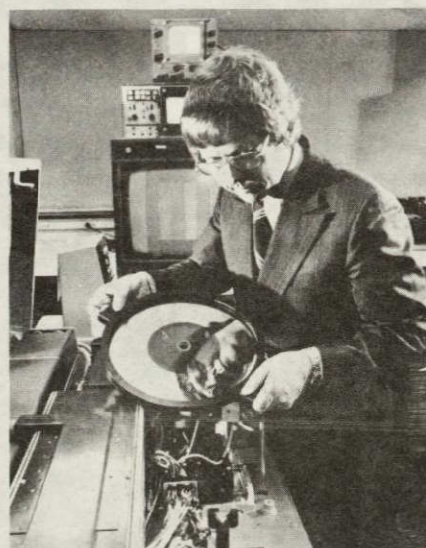
Lee Hedlund, RCA project engineer, loads company's developmental video recording system that is capable of storing 10,000 TV pictures on a one-inch band of the disc.
