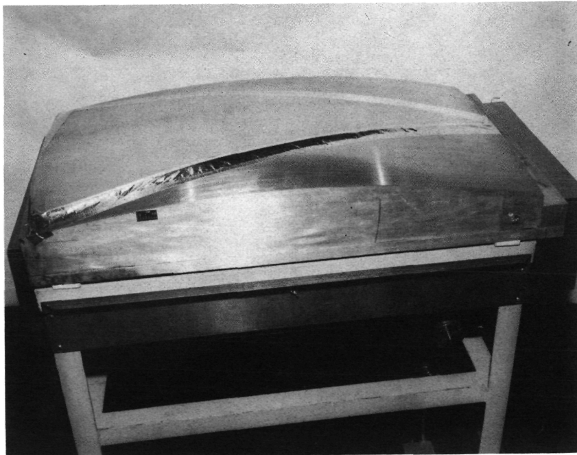
Figure 8. - Concentrator segment taped to forming die.
