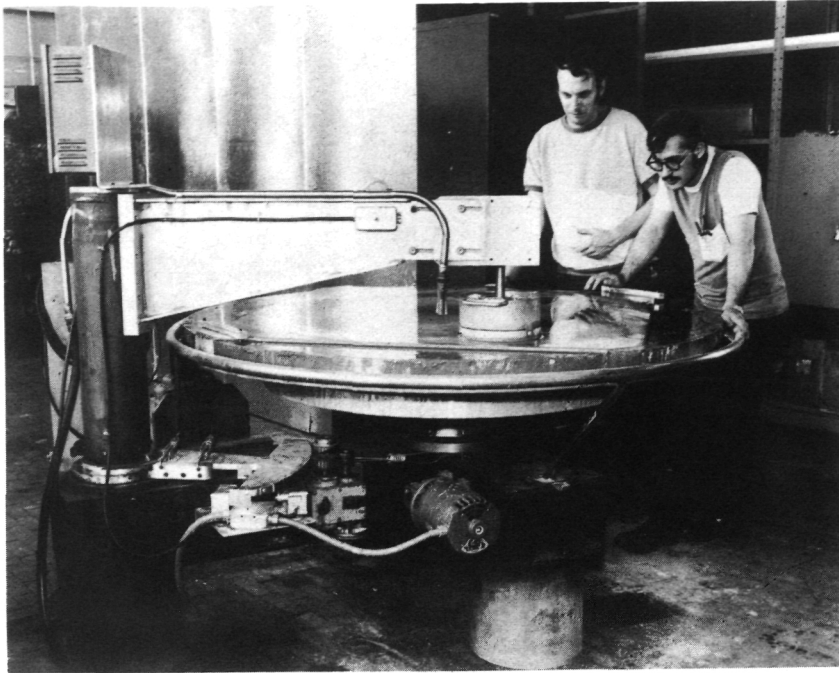
Figure 7. - Polishing of concentrator segment.
