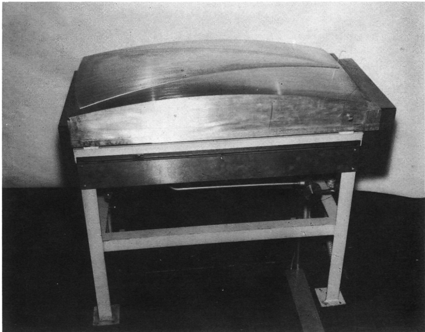
Figure 6. - Petal-forming die with attached distribution sheet.
