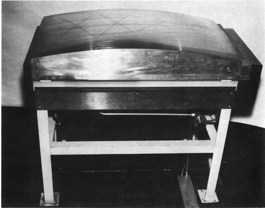
Figure 5. - Petal-forming die complete with heaters, thermocouples, and vacuum slots.
