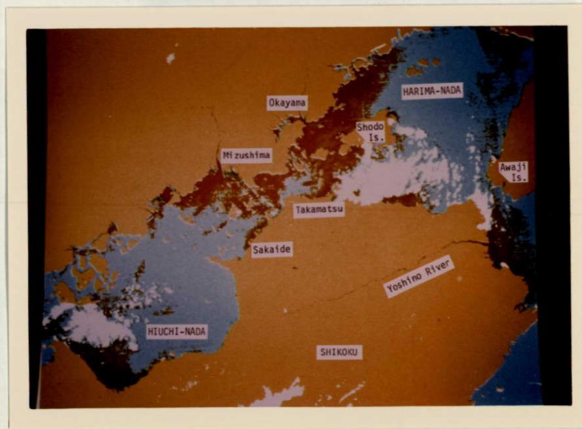
Fig. 3 Patterns of turbid water in the Harima-Nada sea and the Hiuchi-Nada sea extracted from LANDSAT-1's MSS imageries taken on Nov. 12, 1972.
