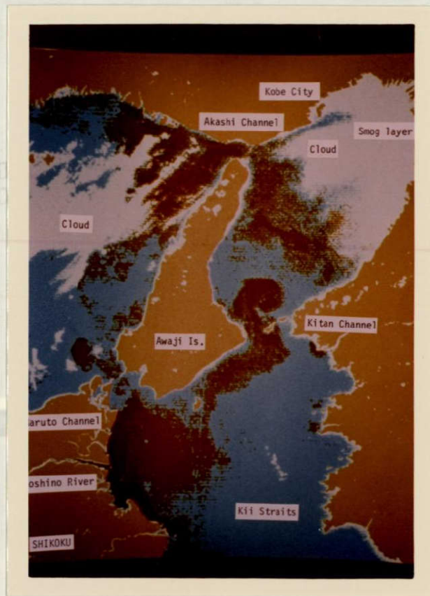
Fig. 2 Patterns of turbid water in the Osaka Bay, the Kii Straits and the eastern part of the Harima-Nada sea extracted from LANDSAT-1's MSS imageries taken on Oct. 24, 1972.
