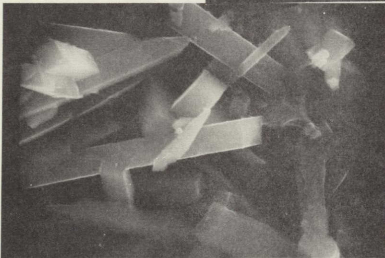
Figure 5. Scanning Electron Micrographs of a Fractured Surface of an MV20 Sample that had been Immersed in HF to Leach the Glass Phase to a Depth of Approximately One-Third the Specimen Thickness.
