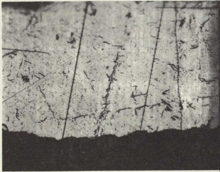
Figure 14. Silicon-Ceramic Interface Carbonized with Dag 154 (500x)
