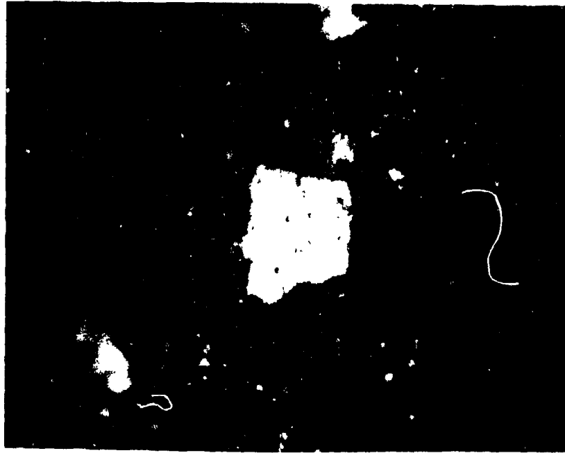
Fig. 15: White clast from 10060,5. Width of field 7.3 mm (S-76-25890)
