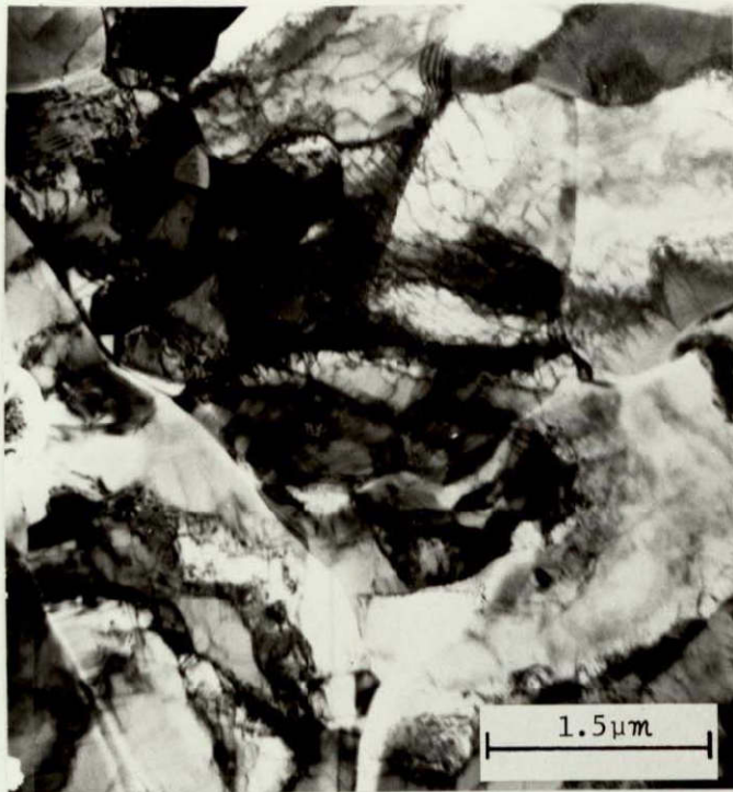
Foil Orientation \langle 110 \rangle (a) Fe-12Ni alloy
