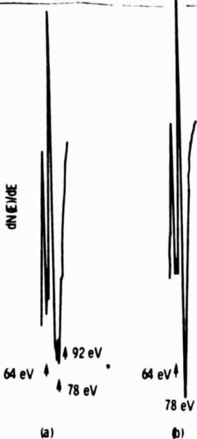
Figure 3. Si LVV Auger peak (a) after Ar^+ bombardment and (b) after O_2^+ bombardment.
