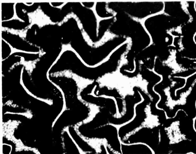
Figure 3. - Sputtered molybdenum disulfide on polycrystalline copper in the final state of film formation, with blistering. X40.
