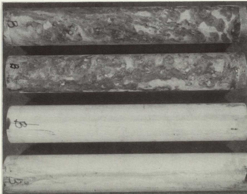
Figure IV-27. Appearance of Task II Tube Specimens After 15 Days Exposure to CASS Corrosion Test.
