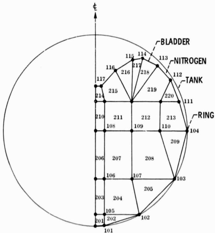
Figure 4. - Model 4 of mercury propellant tank system.
