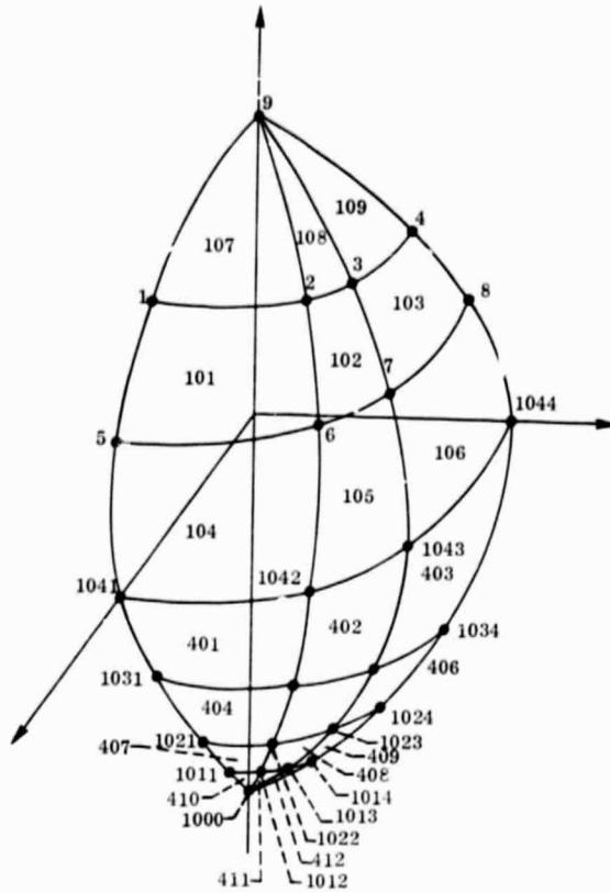
Figure 7. - One quarter model of stainless steel tank.
