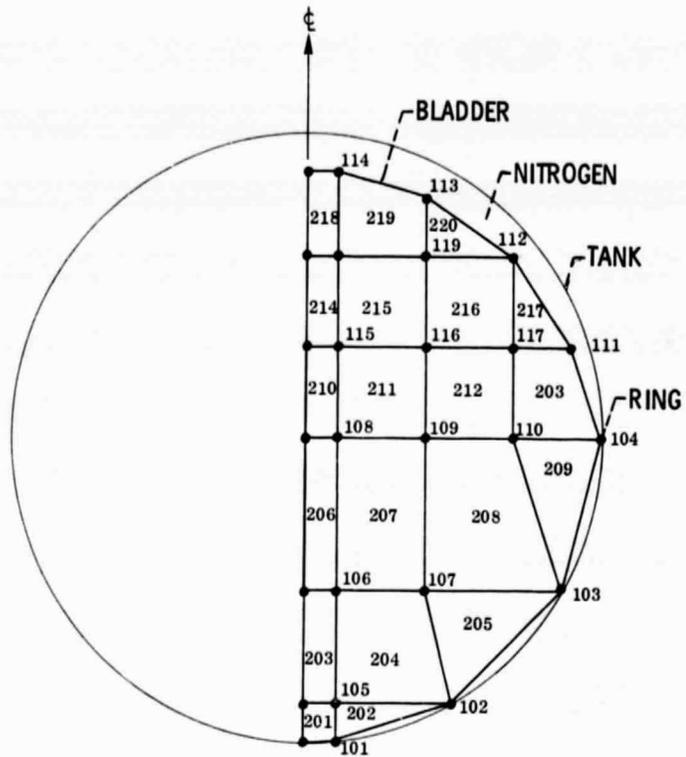
Figure 1. - Model 1 of mercury propellant tank system.
