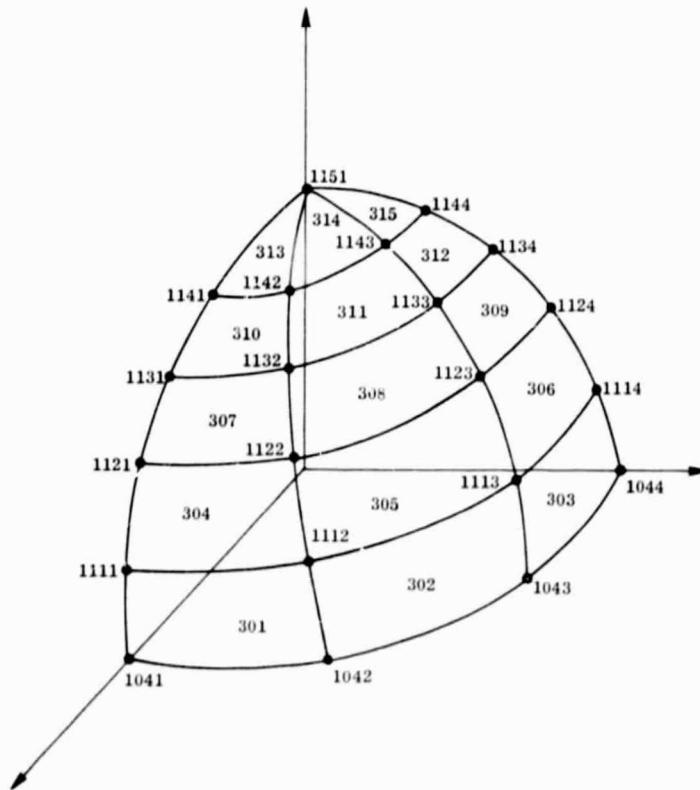
Figure 8. - One quarter model of elastomeric bladder for model 1.
