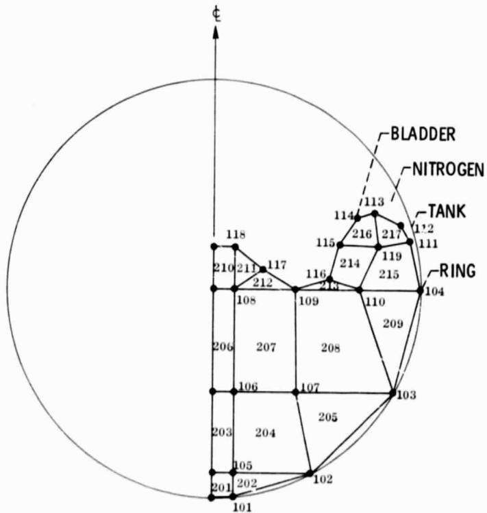
Figure 6. - Model of mercury propellant tank system.
