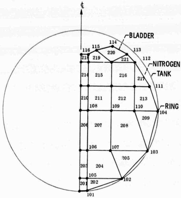
Figure 3. - Model 3 of mercury propellant tank system.
