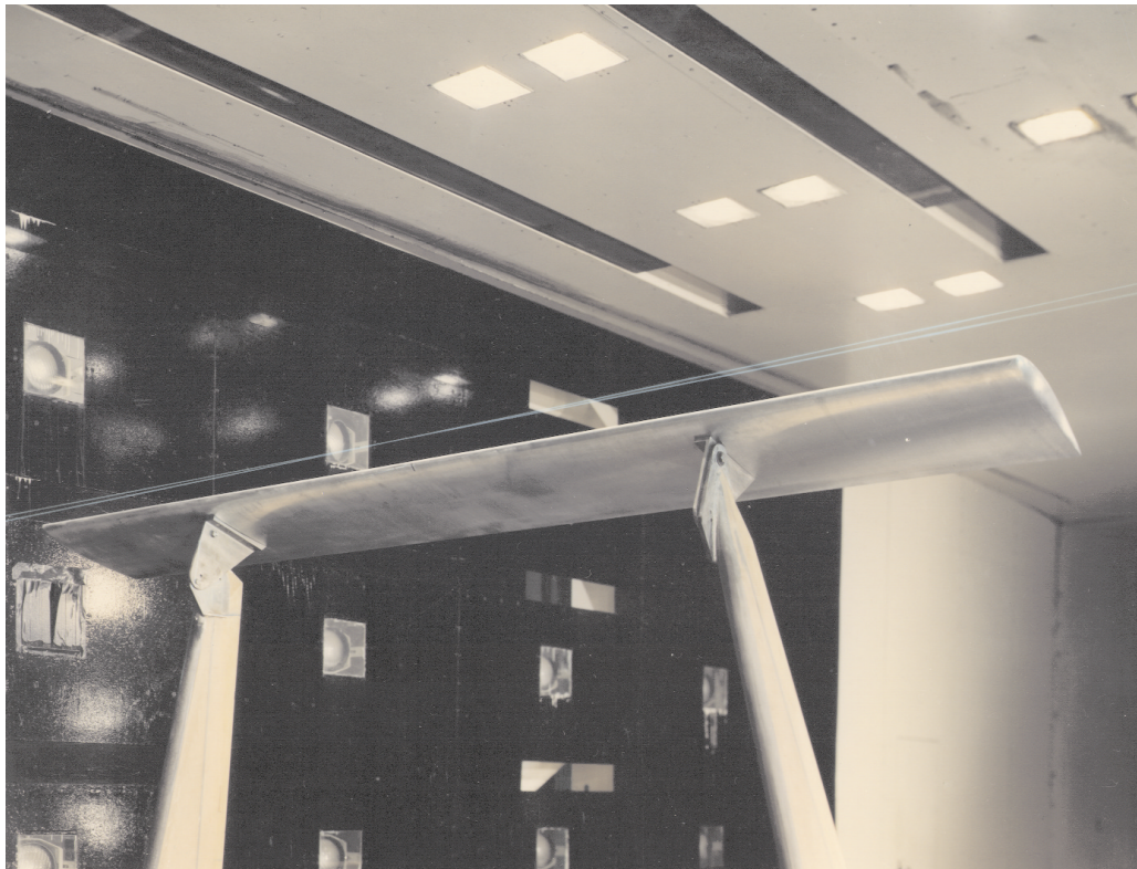
Figure 5.- NACA 0012 wing installed in Langley V/STOL tunnel.
