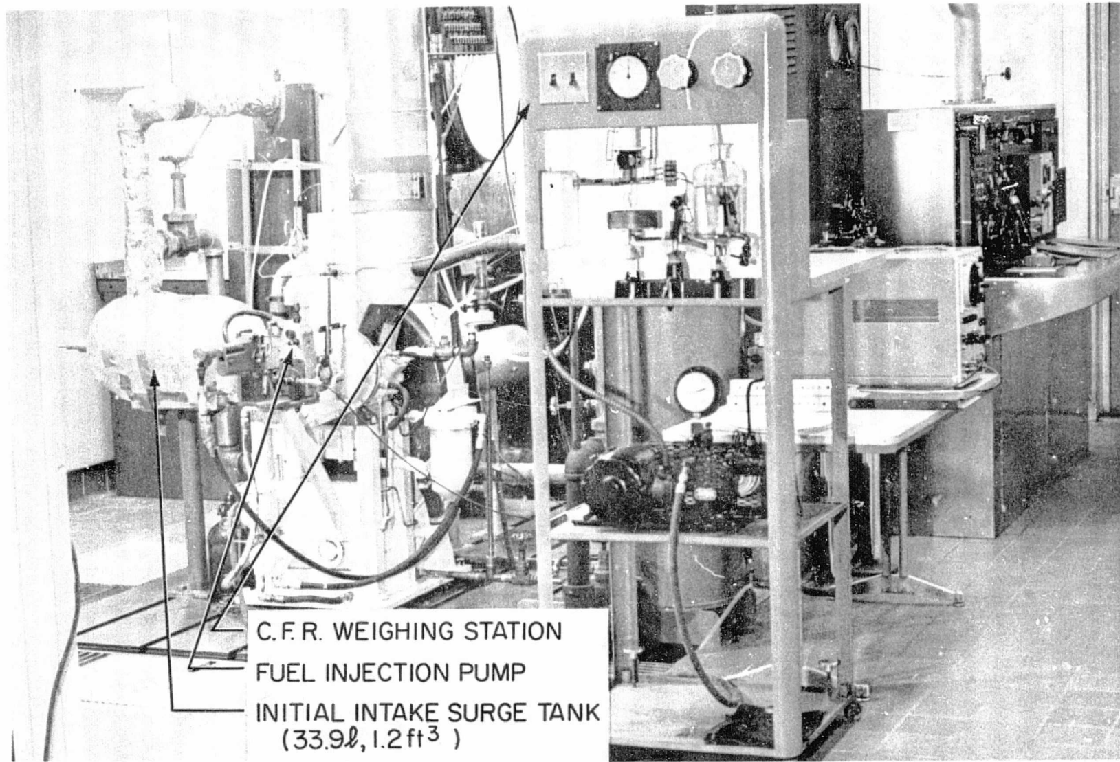
Figure 5. View of Test Installation from Fuel Weighing Station
