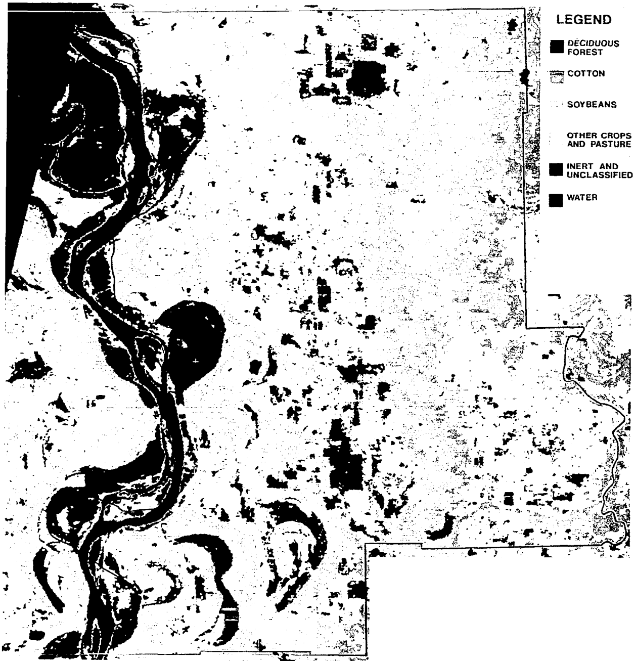
Figure 5.- Computer-implemented classification of Landsat digital data for the demonstration area, reproduced at a scale of 1:62 500.
