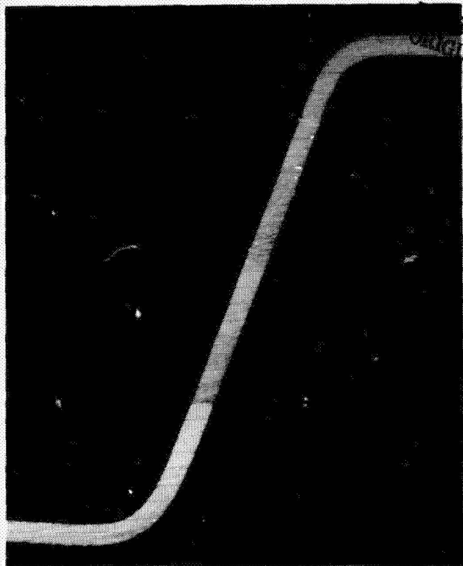
Figure 5-5. — René 41 corrugation bend area enlargement.
