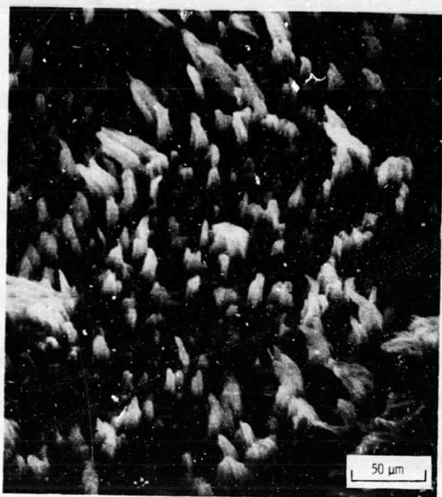
Figure 3. - Argon-ion textured polytetrafluoroethylene, 3000X.
