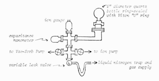
Initially, the ion pump was a large Vac-Ion pump which had pumped our H-10 hydrogen maser standard, and the variable leak was a Granville-Phillips servo valve controlled by the signal from the capacitance manometer. Using this system, one storage bottle was coated by the following procedure:
