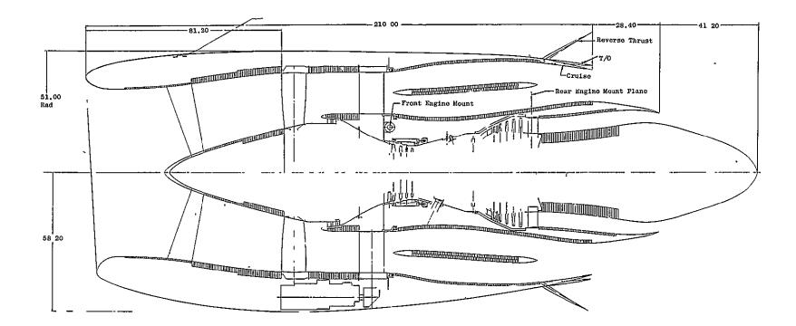
Figure VI-4. Task II GE19/F6E Installation.
