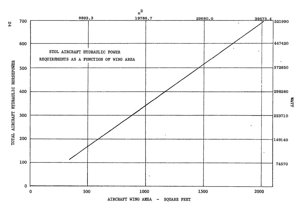
Figure I-1. Task II Requirements, Hydraulic Horsepower.
