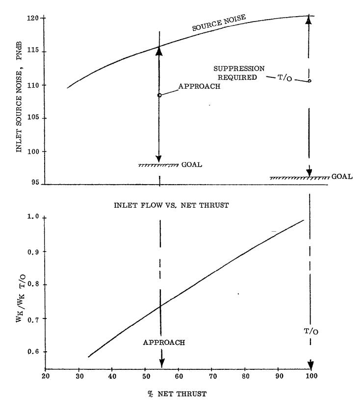
Figure VI-31. Task II GE19/F9 Inlet Suppression and Airflow Characteristics. 272
