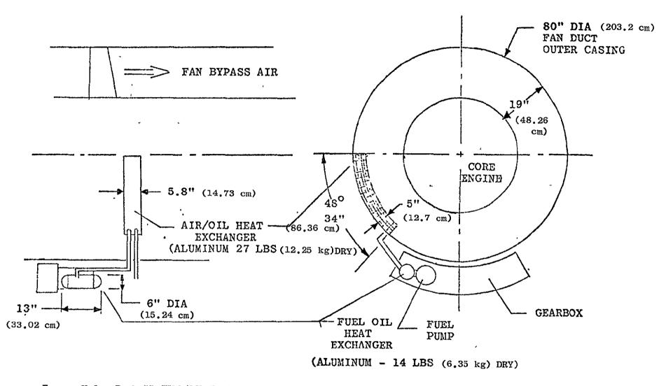
Figure V-3. Task II GE19/F6D Preliminary Size and Installation of Duct Ram Air/Oil Heat Exchanger and Fuel/Oil Heat Exchanger.
