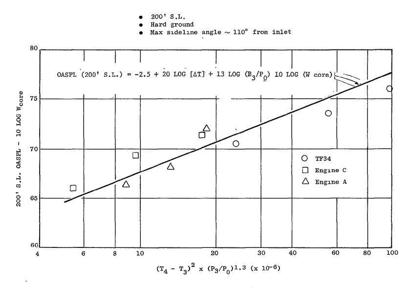
Figure IV-2. Low Frequency Core Noise Prediction Procedure.
