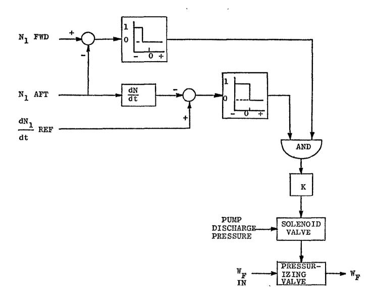
Figure II-11. Task II LPT Overspeed Shutdown System.
