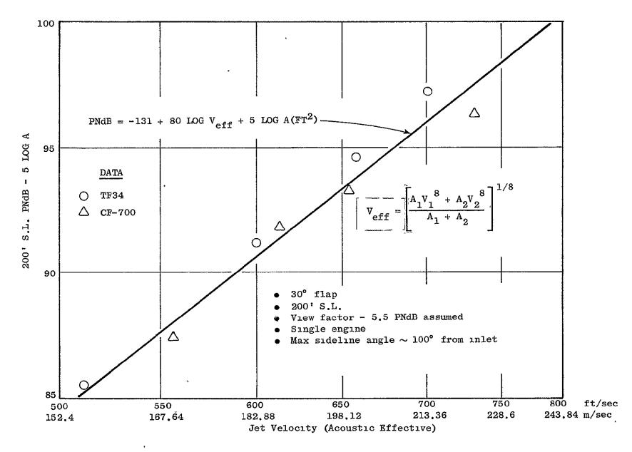
Figure IV-3. EBF Under-the-Wing Flap + Jet Noise Prediction.
