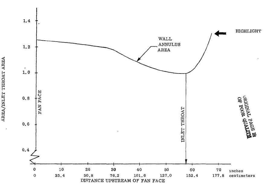
Figure VI-10. Task II F2C Inlet Area Distribution, Throat Area = 3005 inch<sup>2</sup> (3011.5 cm<sup>2</sup>).
