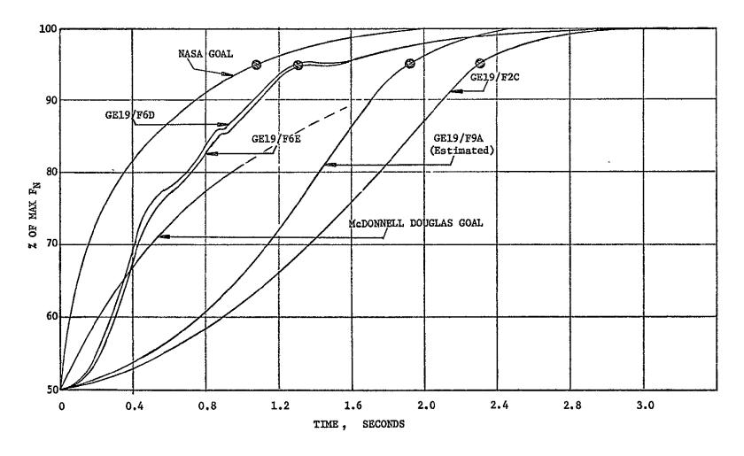
Figure II-13. Task II Transient Responce, Sea Level, 90° F, 100° F  $\Delta T_{41}$  Overshoot.
