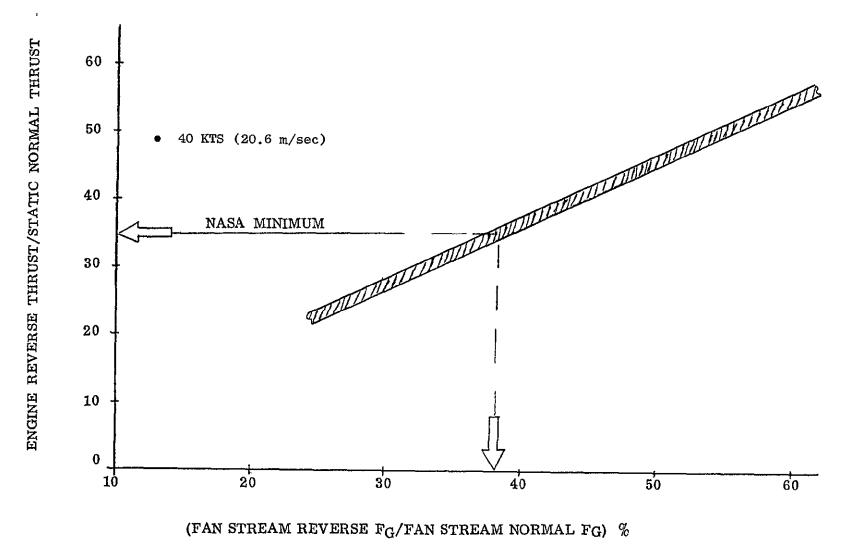
Figure VI-25. Task II VP Reverse Thrust Capability Trends.
