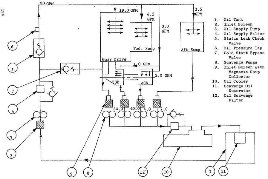
Figure V-2. Task II Geared Fan Lube System.
