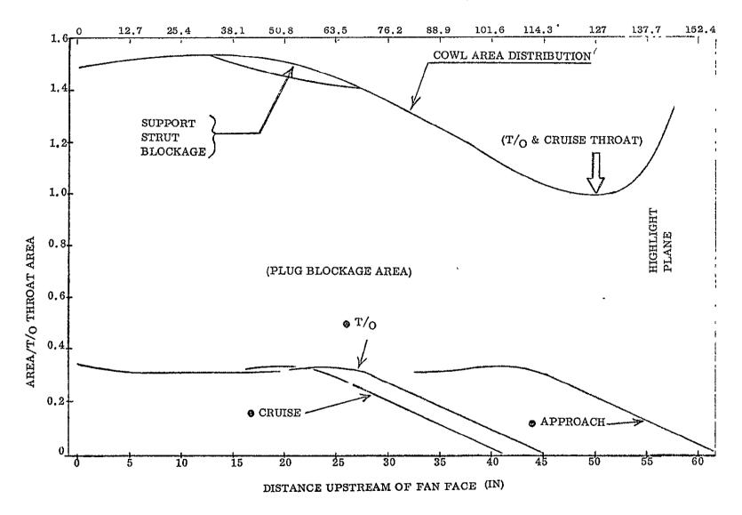
Figure VI-35. Task II GE19/F9A3 Inlet Area Design Factors, T/O and Cruise Inlet Throat Area  $\approx 1080 \text{ inch}^2$  (6967.7 cm<sup>2</sup>).
