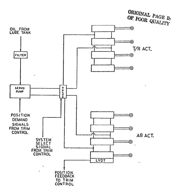
Figure II-8. Task II GE19/F2C (OTW) and F9A Nozzle and Thrust Reverser System.
