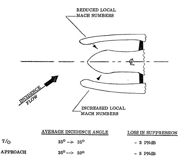
Figure VI-33. Task II GE19/F9A3 Inlet Installation Aero Design Considerations.
