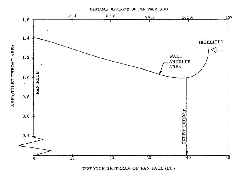
Figure VI-27. Task II GE19/F9A2 Inlet Area Distribution, Throat Area  $\approx$  1120 inch<sup>2</sup> (7225.8 cm<sup>2</sup>).
