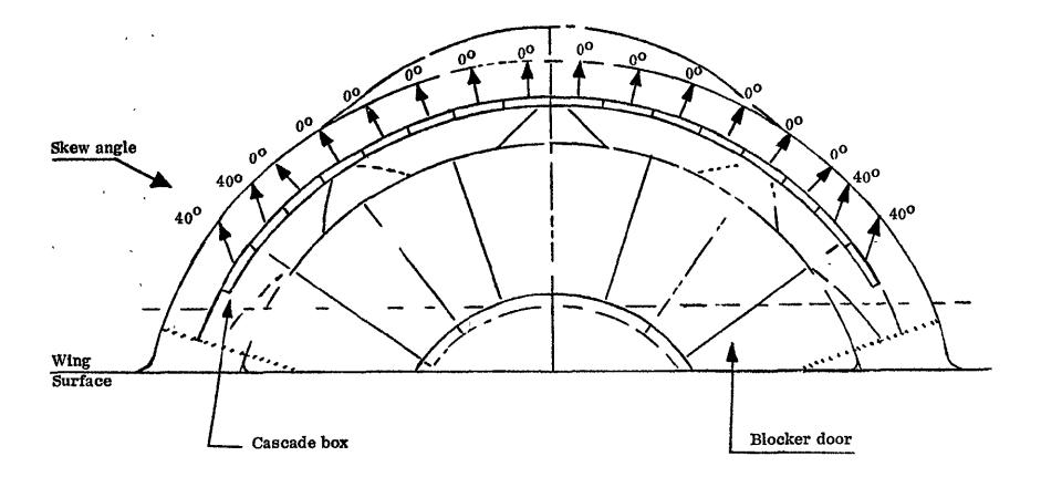
Figure VI-19. GE19/F2C3 (OTW) Reverse Flow Efflux Pattern.
