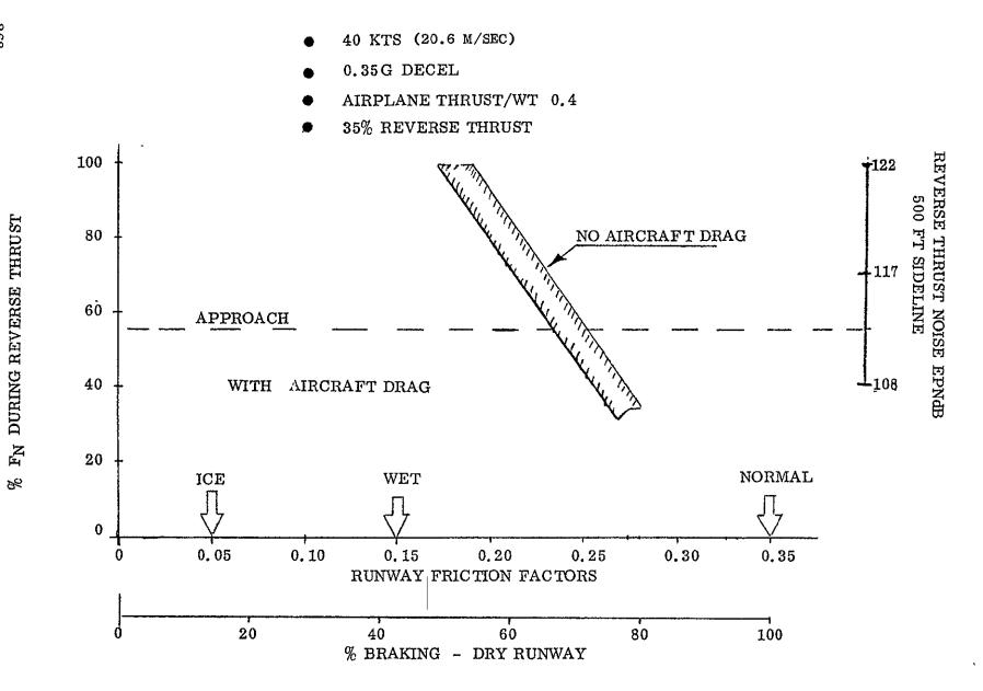
Figure VI-29. Task II AW Reverse Thrust, Noise, and Aircraft Braking Trades.
