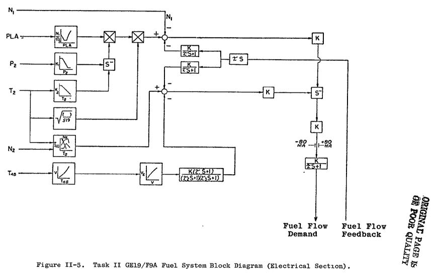
Figure II-5. Task II GE19/F9A Fuel System Block Diagram (Electrical Section).
