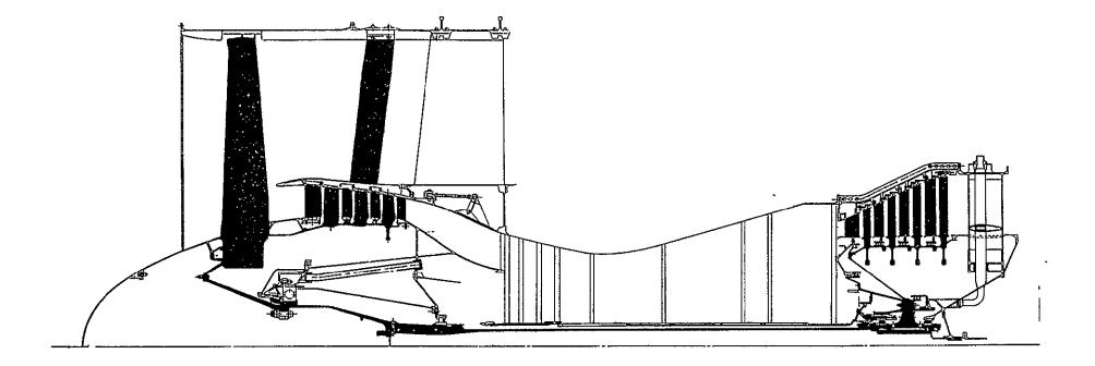
Figure S-3. GE19/F2C Cross Section.
