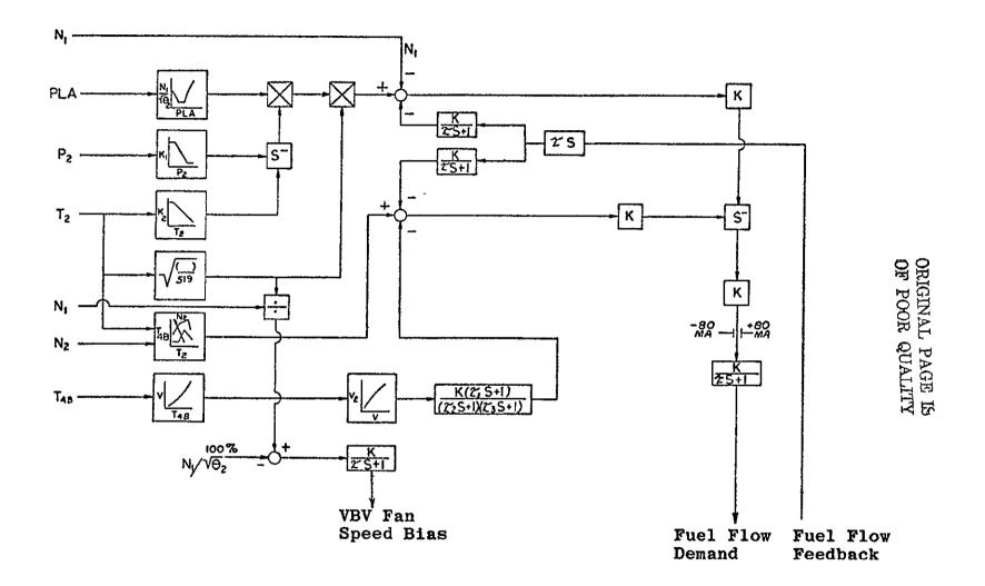
Figure II-3. Task II GE19/F2C and F6 Fuel System Block Diagram (Electrical Section).
