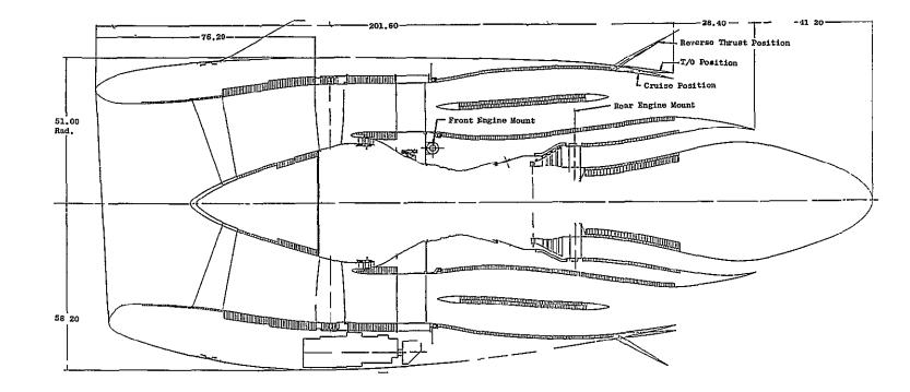
Figure VI-5. Task II GE19/F6D Installation.
