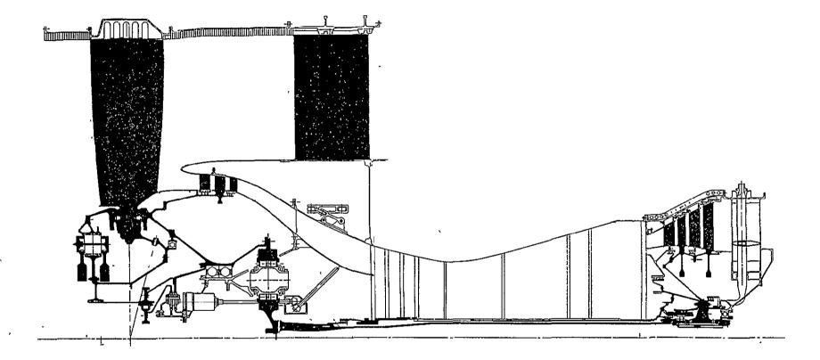
Figure S-4. GE19/F6D Cross Section.
