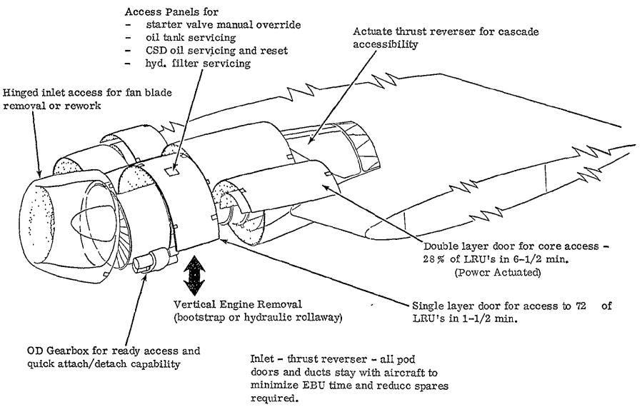
Figure VII-8. GE OTW Engine on Wing Maintainability, Detailed.
