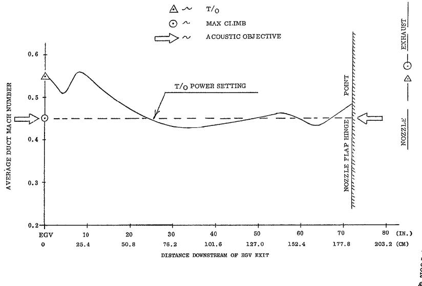
Figure VI-23. Task II GE19/F6 Fan Exhaust Average Mach Number Distributions.
