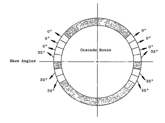
Figure VI-30. GE19/F9A2 & A3 (AW) Reverse Flow Efflux Pattern.
