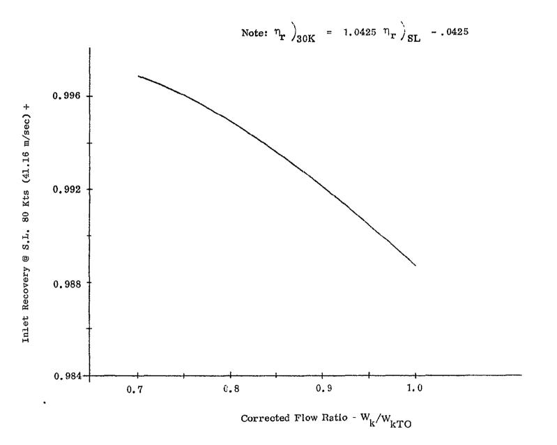
Figure VI-28. GE19/F9A2 Inlet Recovery Vs. Corrected Flow.
