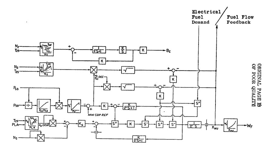
Figure II-6. Task II GE19/F9A Fuel System Block Diagram (Hydromechanical Section).
