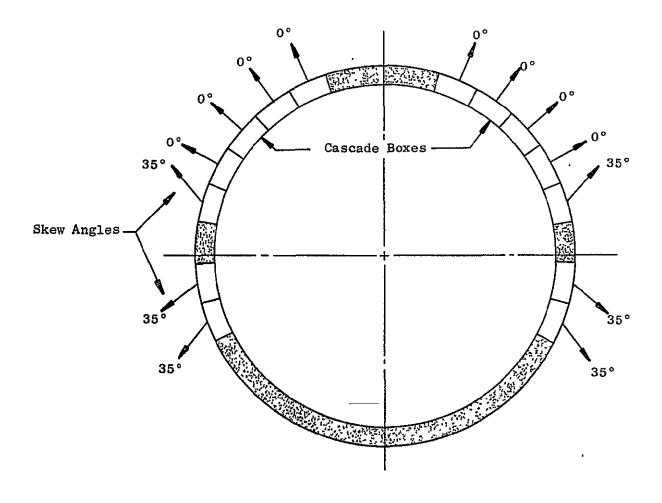
Figure VI-14. GE19/F2C1 & C2 (EBF) Reverse Flow Efflux Pattern.
