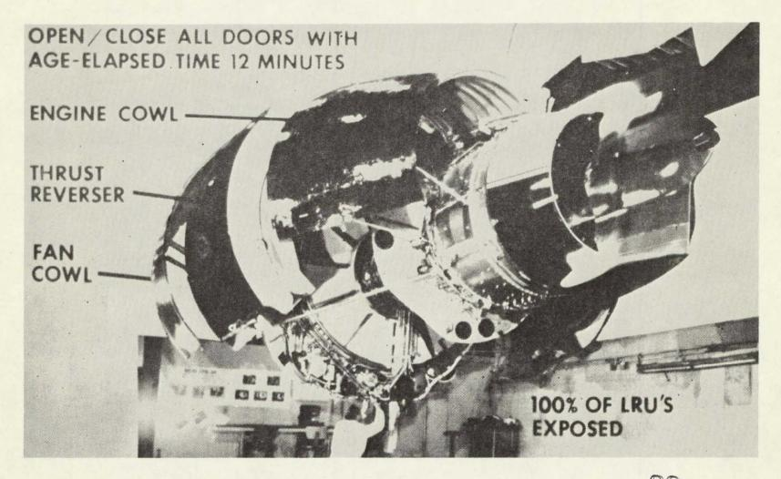
Figure VII-3. CF6 Nacelle Quick Access.
