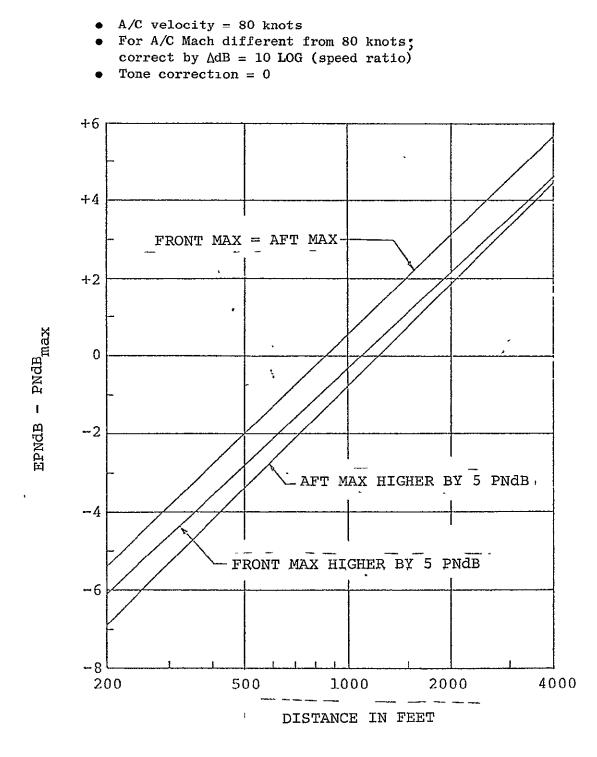
Figure IV-1. Approximate PNdB to EPNdB Conversion for Highly Suppressed Engines.
