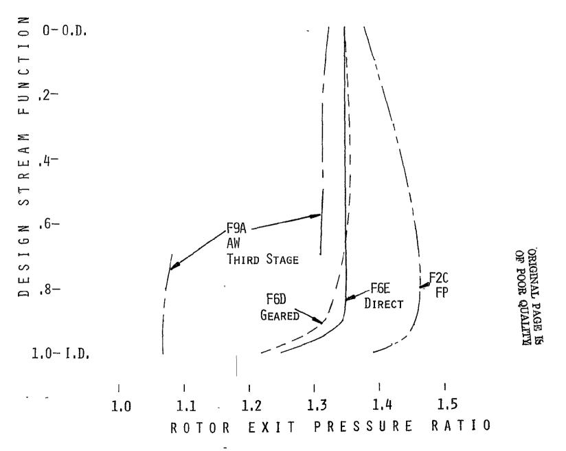
Figure I-12. Task II Radial Distribution of Rotor Total Pressure Ratio.
