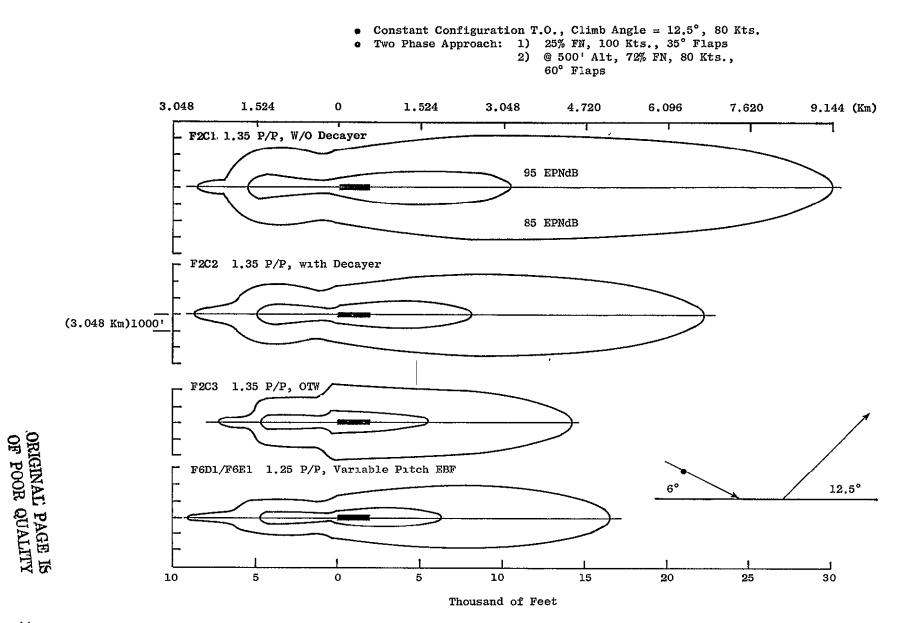
Figure IV-7. Footprint Comparisons (F2C1, F2C2, F2C3, and F6D1/F6E1).
