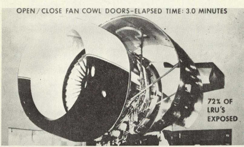
Figure VII-2. CF6 Nacelle, Quick Access.
