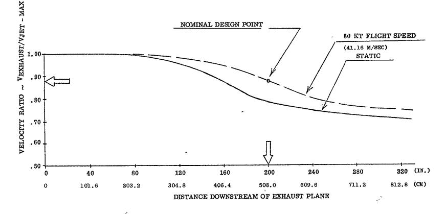
Figure VI-15. Task II GE19/F2C2 Exhaust Velocity Decay Characteristics (Max. Exhaust Velocity Ratio Vs. Distance from Exhaust Plane).
