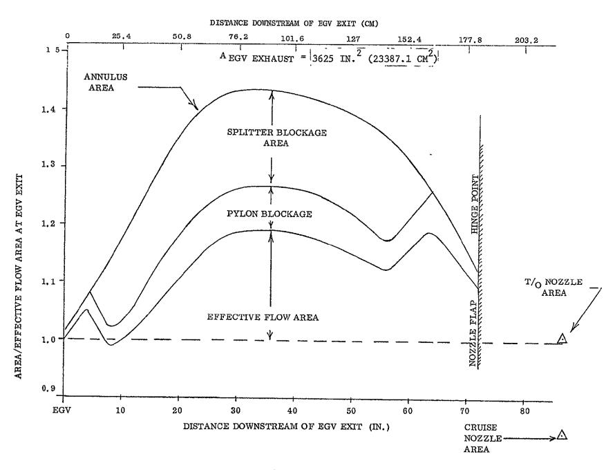
Figure VI-22. Task II GE19/F6 Fan Exhaust Duct Area Distribution.
