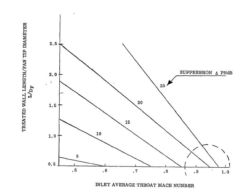
Figure VI-32. Task II GE19/F9A2 Inlet Acoustic Design Trends, Effect of Combined Wall Treatment and High Throat Mach Number on Suppression.
