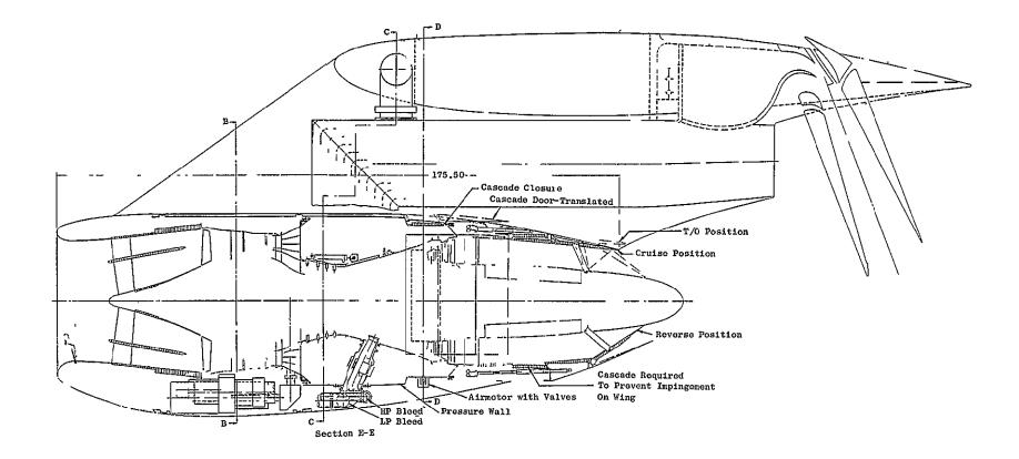
Figure VI-6. Task II GE19/F9A2 Installation.
