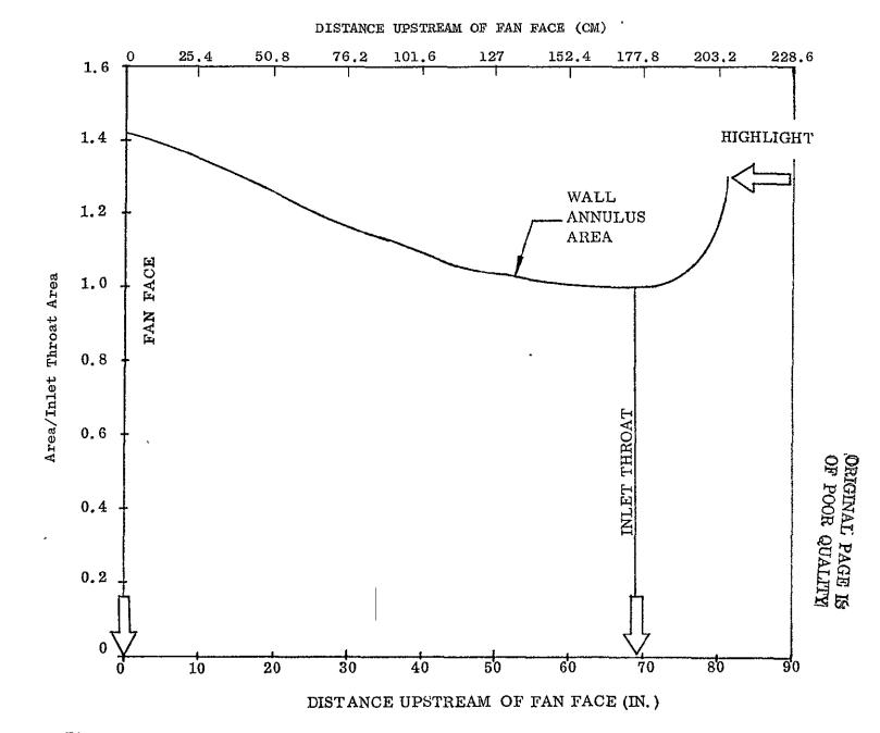
Figure VI-20. Task II GE19/F6E Inlet Area Distribution, Throat Area  $\approx 3830$  inch² (24710 cm²).
