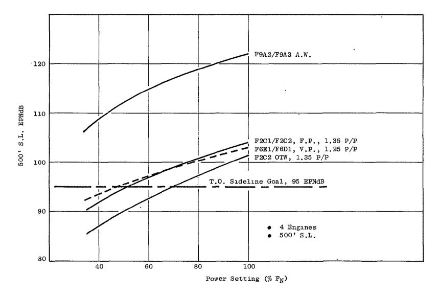
Figure IV-6. Thrust Reverser Noise Level Comparison.
