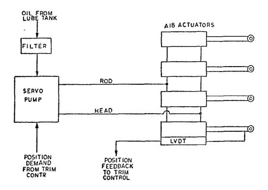
Figure II-7. Task II GE19/F2C and F6 Nozzle Actuation System.
