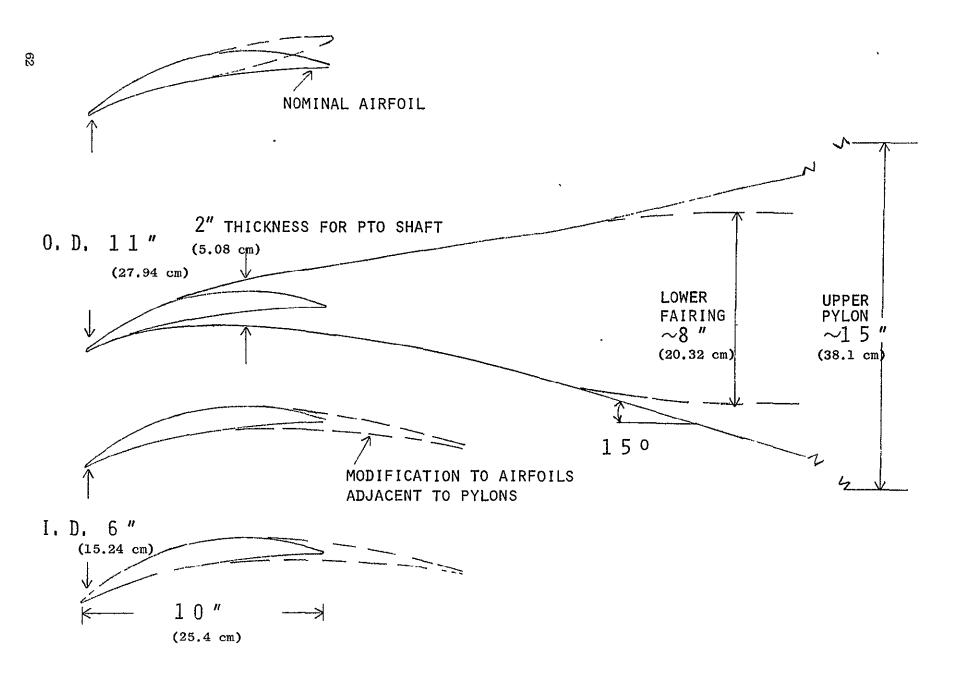
Figure I-14. Task II Vane-Frame for VP Fans.
