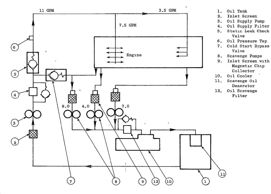
Figure V-1. Task II Direct-Drive Lube System.
