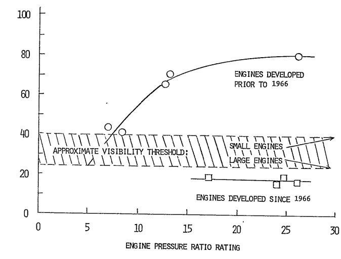
Figure III-1. Comparison of Peak Smoke Emission Characteristics.
