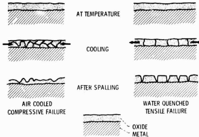
Figure 9. - Schematic representation of the effect of cooling rate on spalling.
