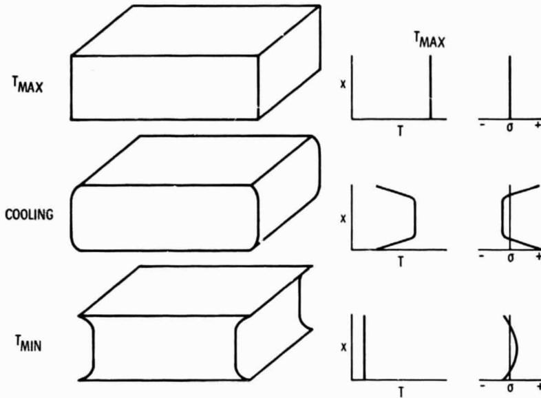
Figure 8. - Thermal shock in a ductile alloy-schematic.
