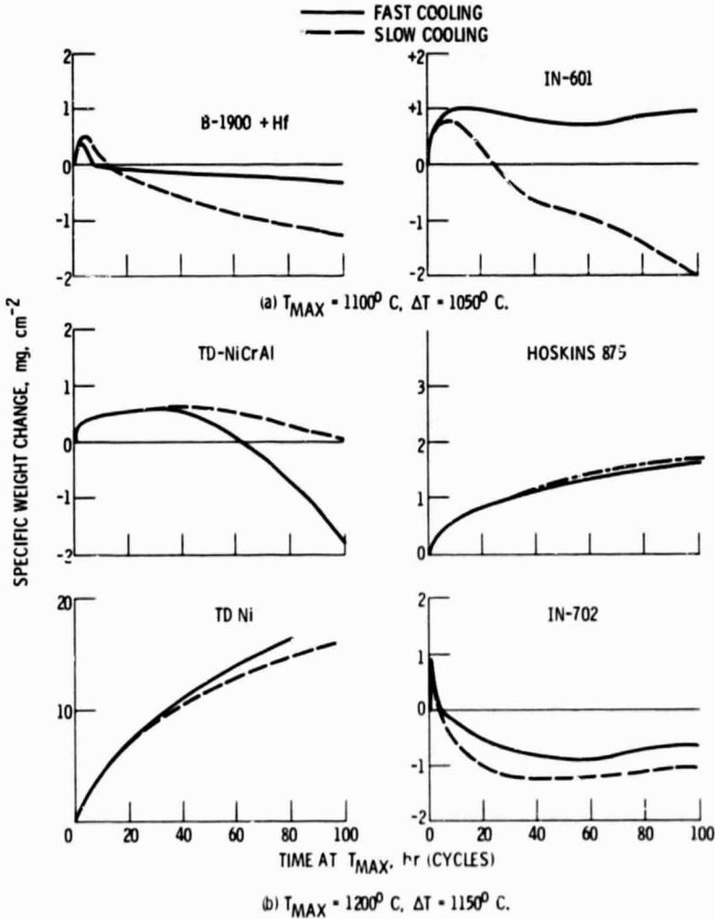
Figure 3. - The effect of cooling rate on the cyclic oxidation of some high temperature alloys, one hour at T<sub>MAX</sub> and one half hour at T<sub>MIN</sub> per cycle.
