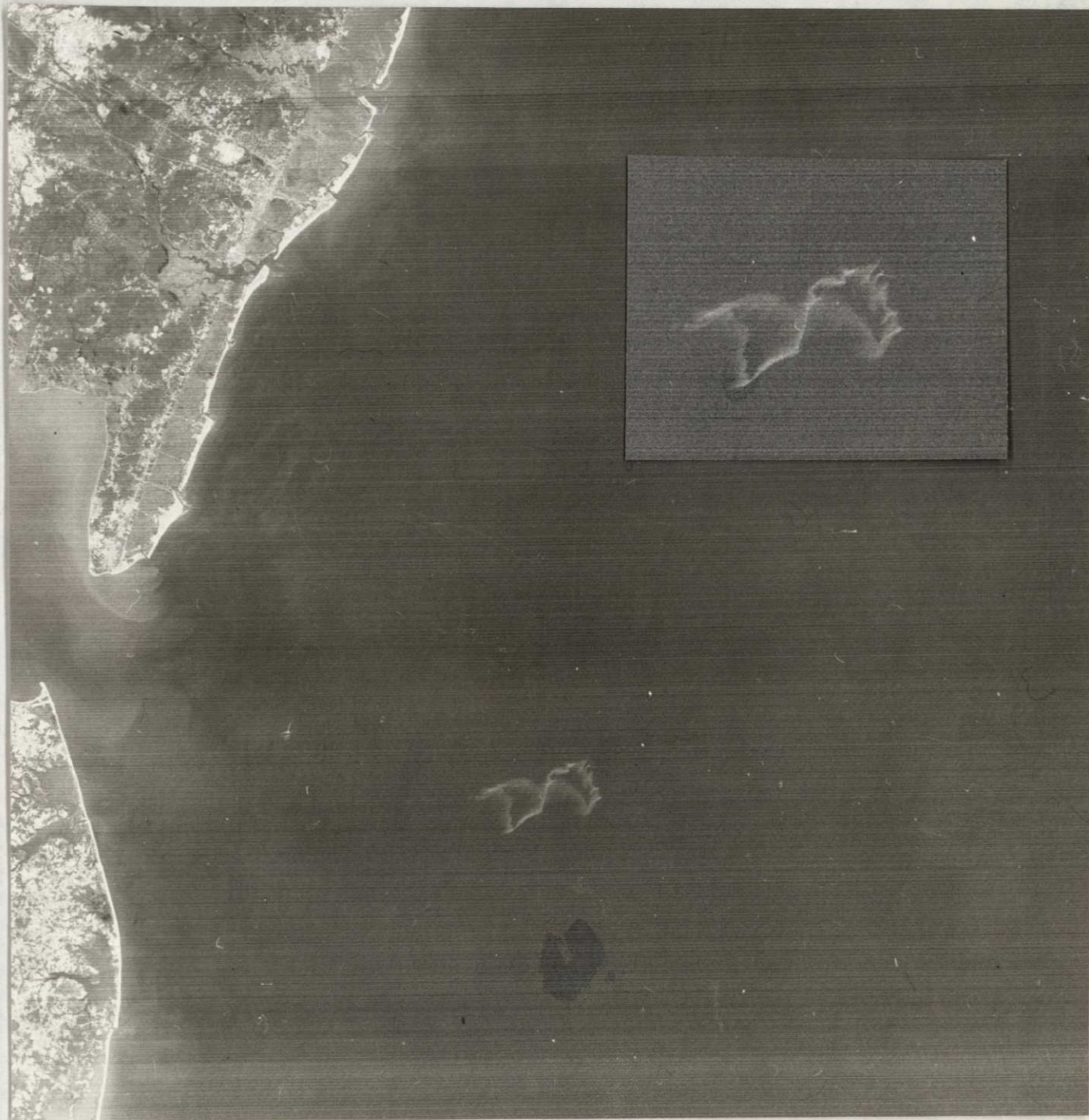
Figure 3.7. Landsat image for 24 February 1976. The insert shows the acid plume and the sites of the training sets.
