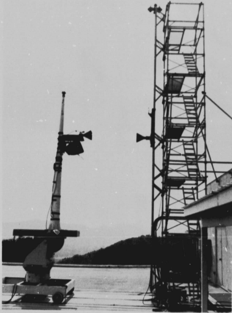
Fig. 2. Test Setup at JPL Antenna Range Facility. Horns are 152.4 cm (5 ft) apart
