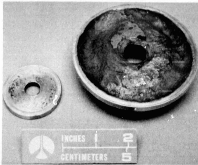
Figure 108. Damaged Turbine Simulation. Orifices
