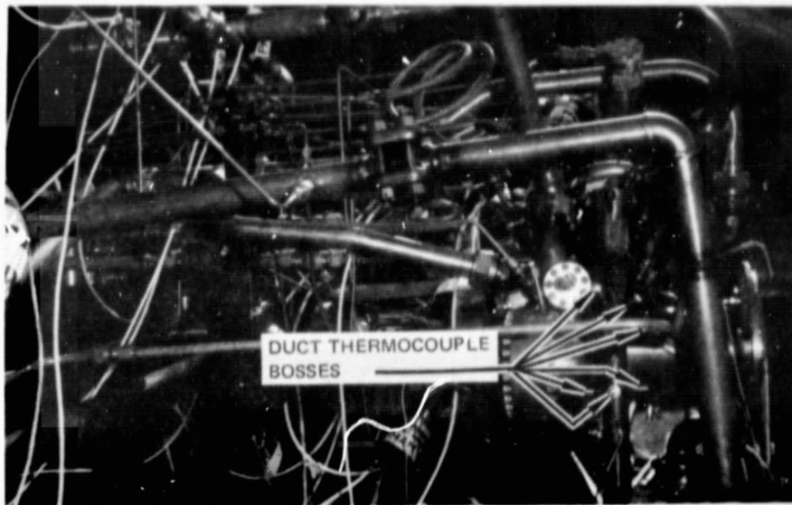
Figure 128. Stage Combustion Assembly Installation With Duct Thermocouple Bosses
