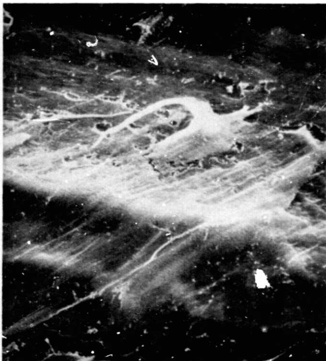
(c) TEFZEL R SPUTTER ETCHED 1.2 HOURS BY 750 eV ARGON IONS AT 0.3 mA/cm 2 .
