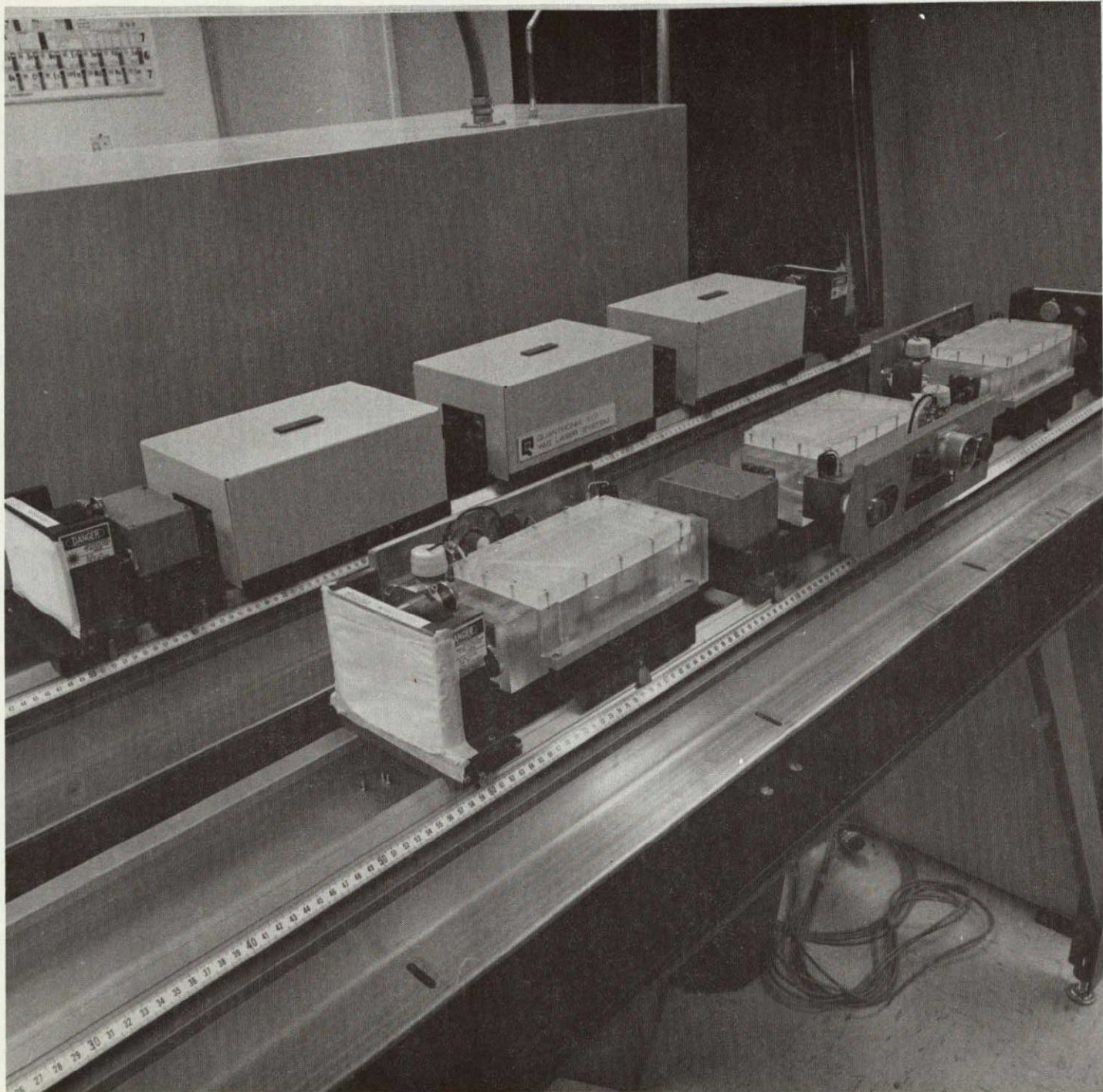
FIGURE 4: Nd:YAG LASER SYSTEMS (2) ON RAILS
