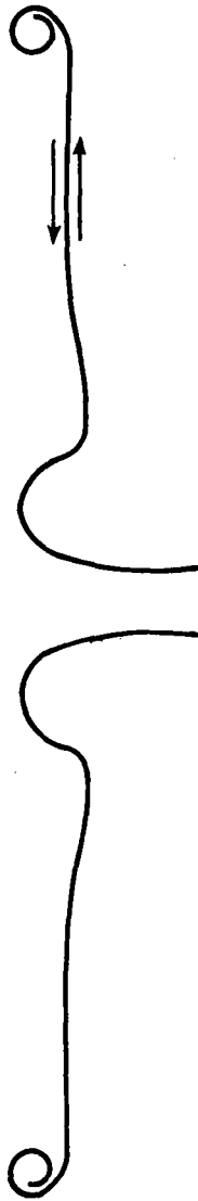
(b) Distributed vortex method. Absence of large local velocities permits the sheet to roll up smoothly.
