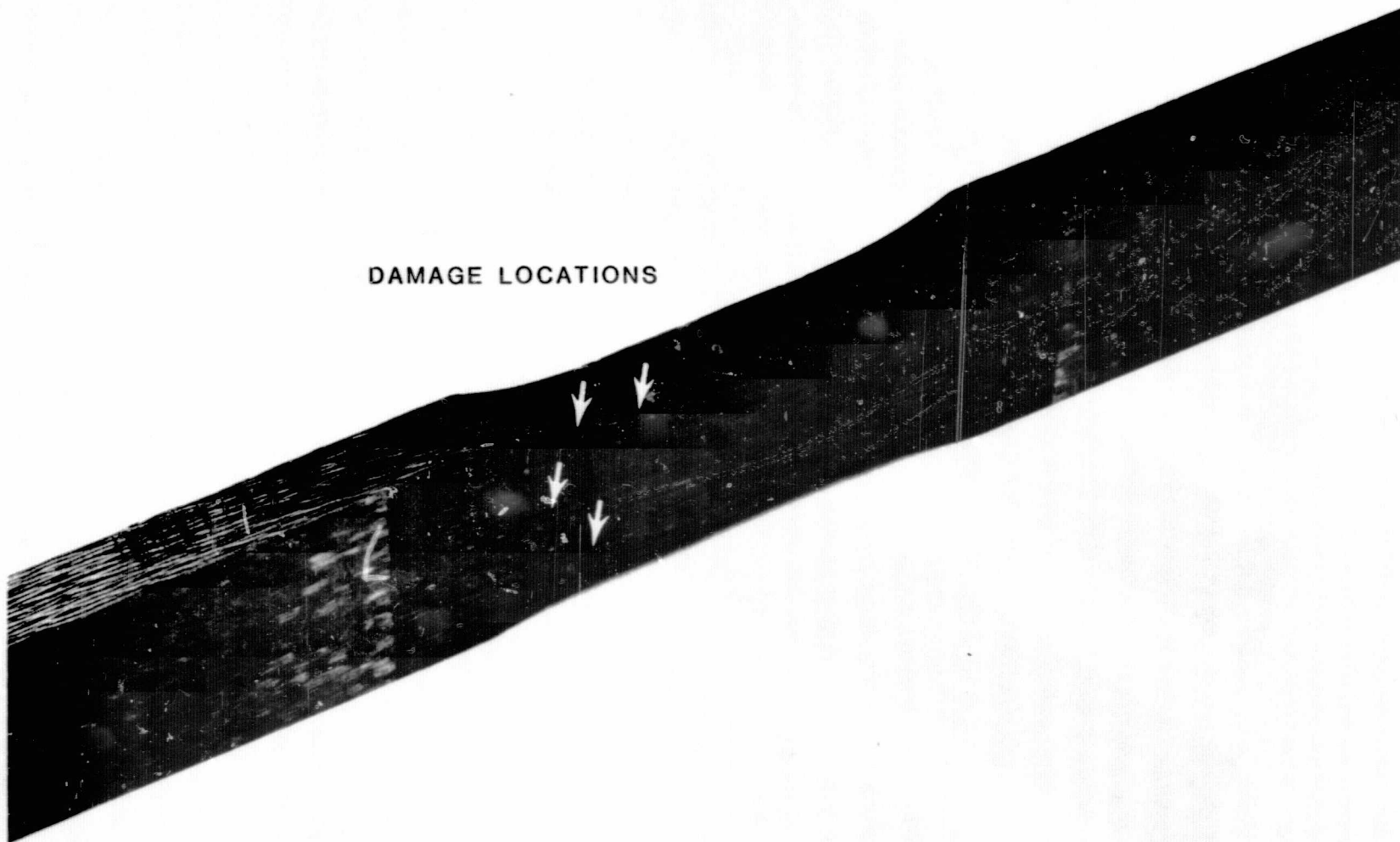
Figure 20. T-300/PMR-15 Fatigue Specimen Showing Typical Damage Locations after Test.
