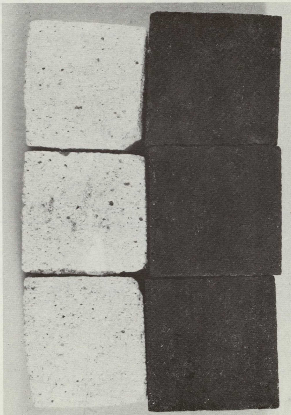
Figure 23. Pre-immersion K14 mortar and carbon brick
