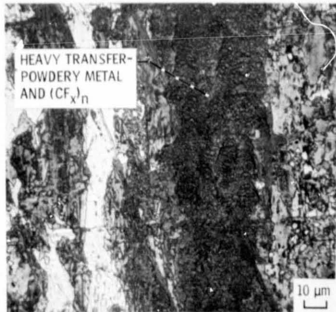
(b) (\text{CF}_x)_n FILM WEAR TRACK
