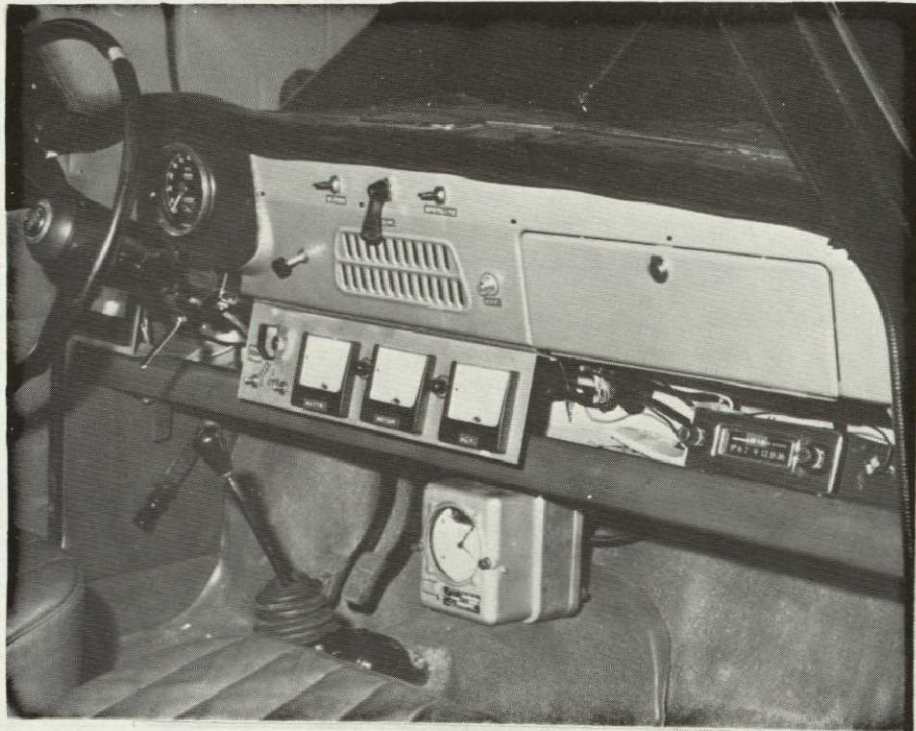
Figure 8. - Location of gages on dashboard of Kordes hybrid.
