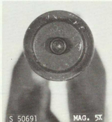
Figure 36 Decrease Solenoid Pintle With the Most Wear
