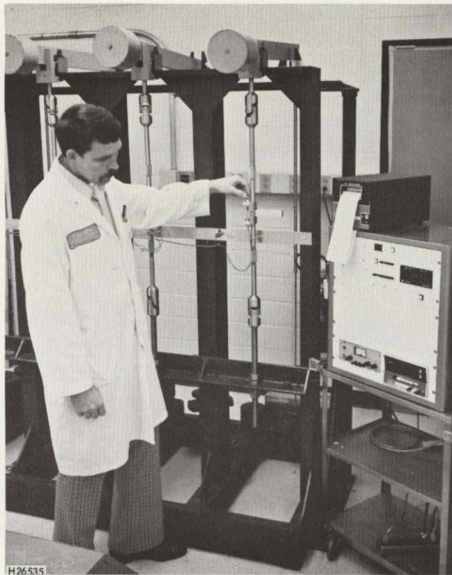
Figure A-1. Direct Load Tests of DCB Specimens
