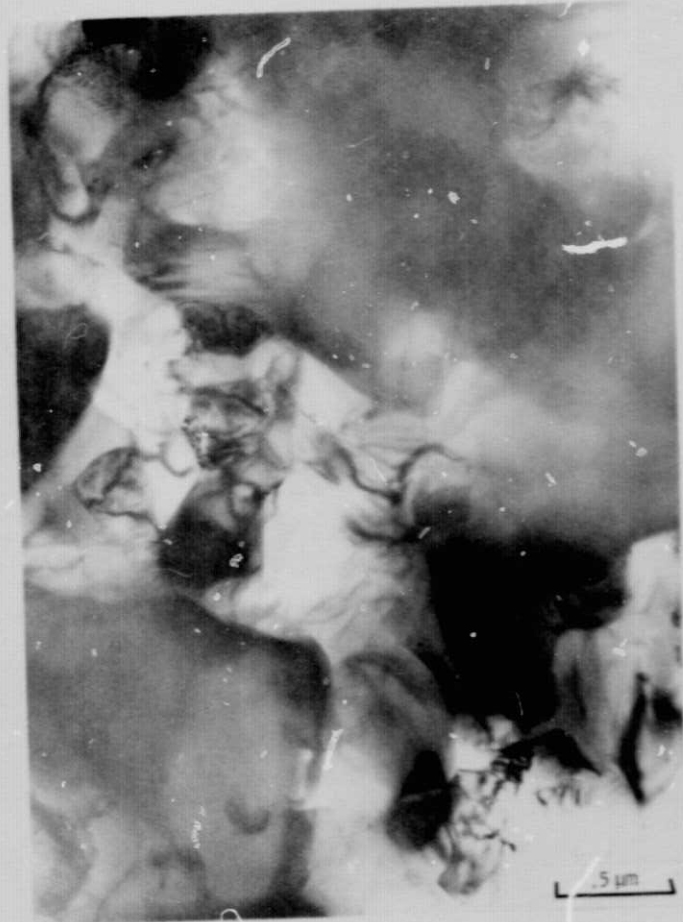
Figure 5. - TEM Micrograph of 60 wt% Al_2O_3 - 40 wt% Si_3N_4 compact hot-pressed at 1550^\circ C , 27 MPa (4 ksi) for 2 hours.
