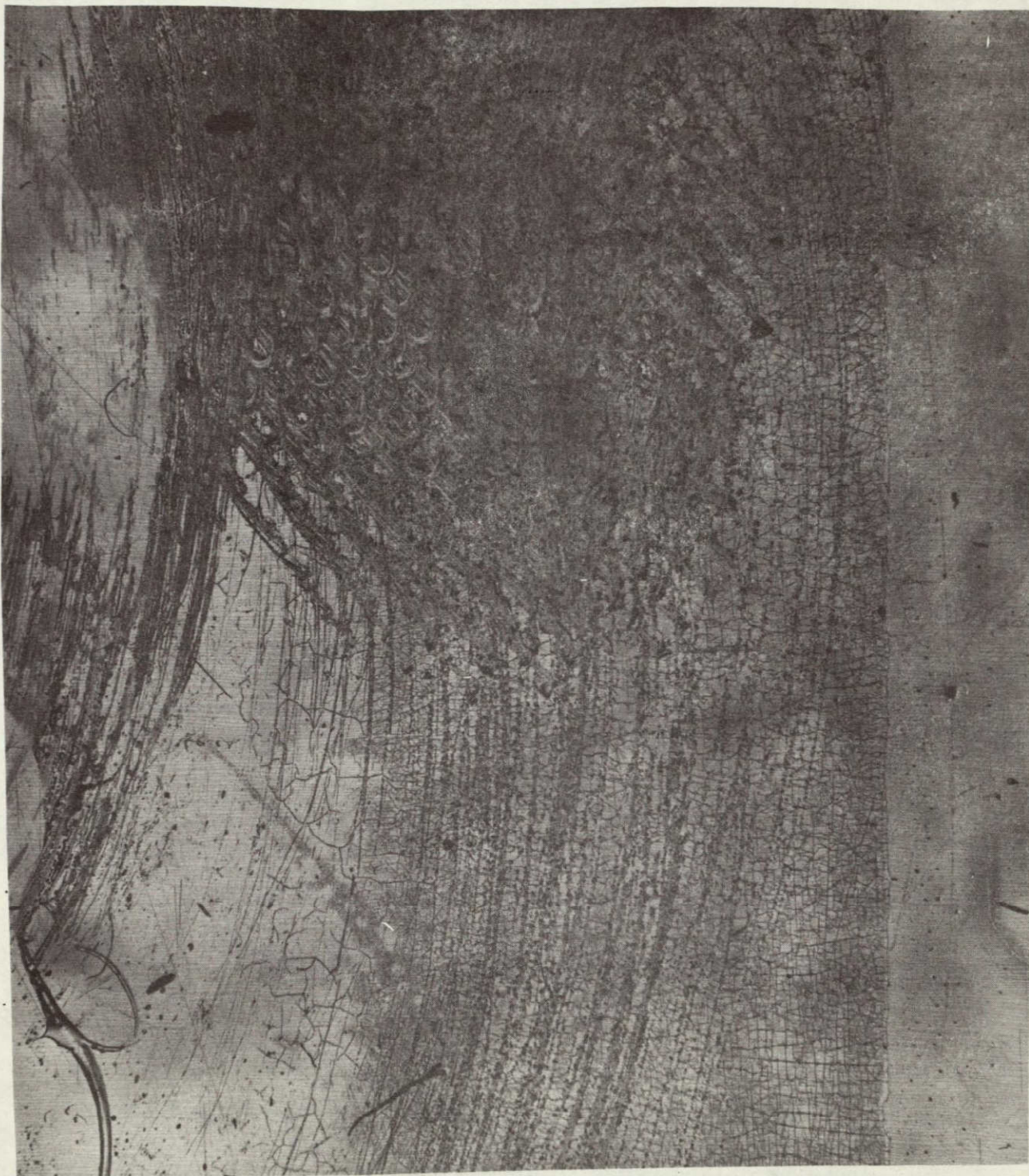
Figure 7 Photograph of Ag/FEP Sample 2C (Area to the Left of Center), 2B (Center Area), 2A (Area to the Right of Center) Contaminated by the CVCM from RTV-560 and Exposed to 2.32 ES. Vertical Streaks are from an Accidental Brush by a Gloved Hand. The Clear Area to the Extreme Right was Covered up by Sample 3C. Magnification 10x.
