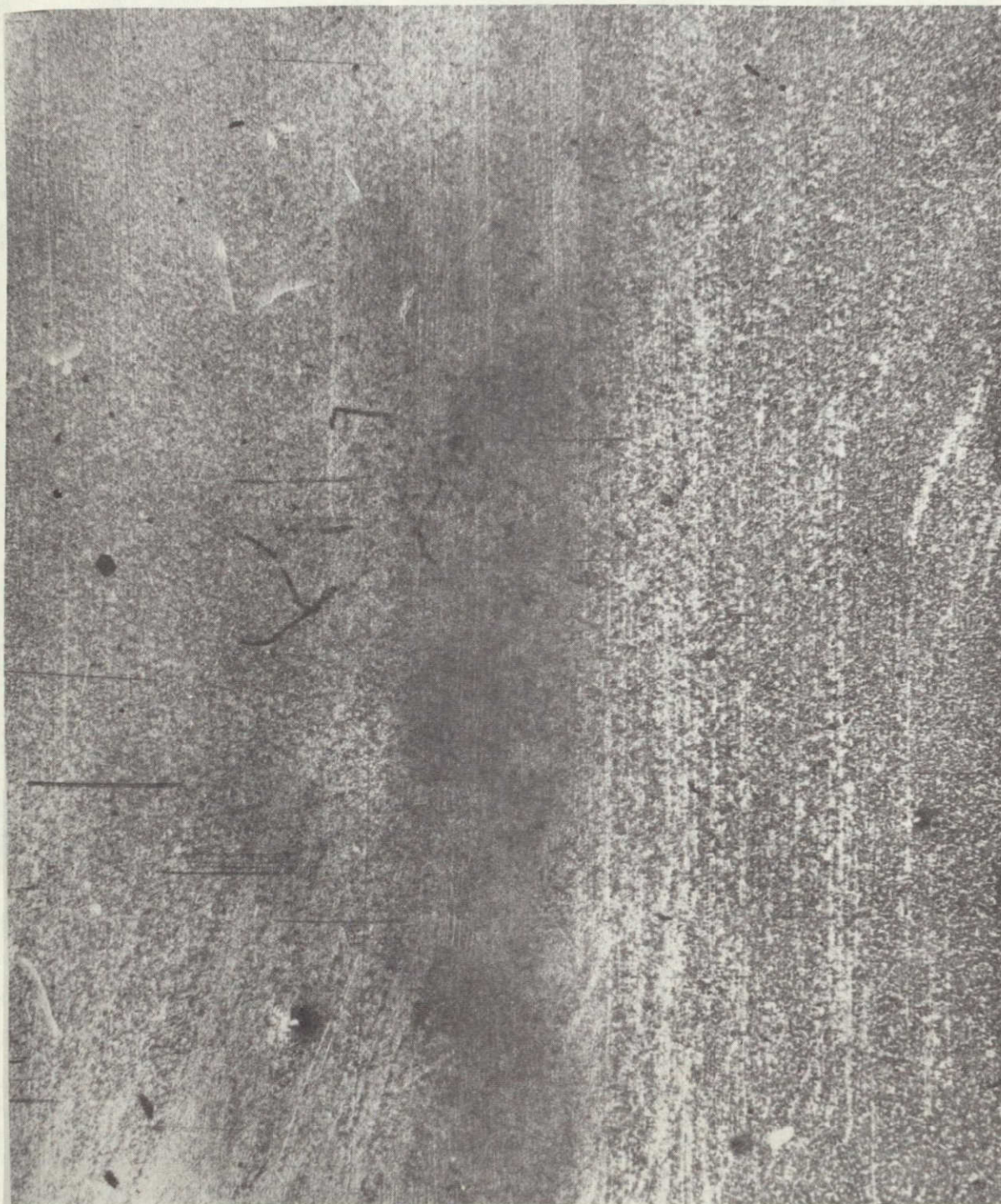
Figure 16 Photograph of Ag/FEP Sample 3 Contaminated by the CVCM from Hydraulic Fluid (Relative Thickness Under Vacuum 574 nm) and Exposed to Vacuum Ultraviolet Radiation 124 nm for 212 Hrs. 25x.
