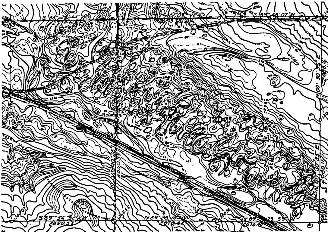
Figure 7.23. Part of U.S. Bureau of Reclamation topographic map of the Columbia Basin Project. The 2-foot contour interval provides an excellent display of the
