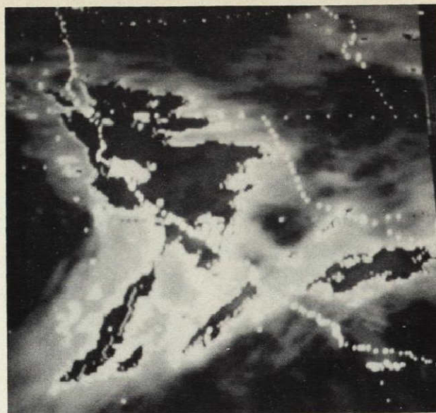
FIG. 8. Enhanced GOES-W IR image from a digital display for 1745 GMT, 15 March 1977, showing a Pacific storm entering the California coastal region. Darker gray represents CTTs from -43^{\circ} to -47^{\circ}\text{C} ; medium gray, from -39^{\circ} to -43^{\circ}\text{C} ; and white, from -31^{\circ} to -39^{\circ}\text{C} .
