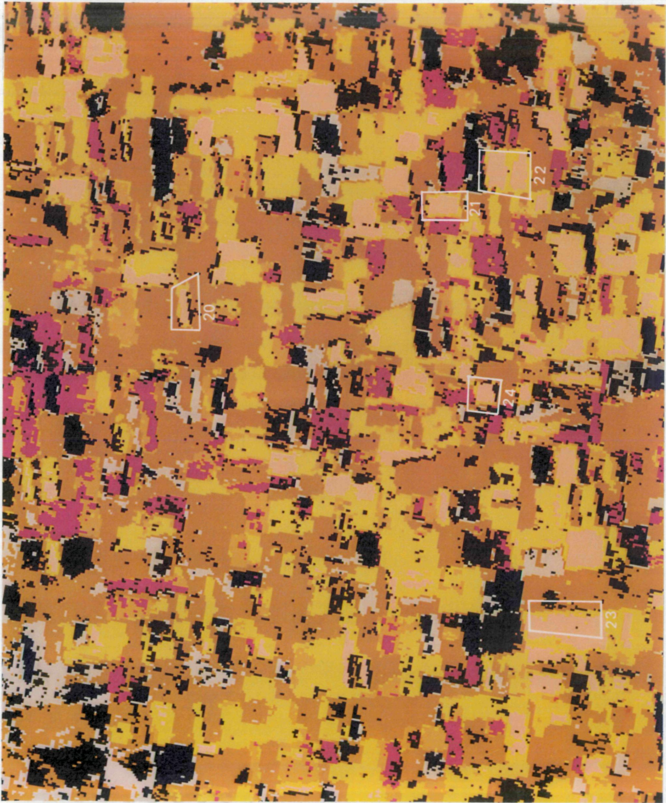
Fig. 3-9 Categorized Imagery - Bendix Restoration 40 x 40 Meter Sampling Interval, Assumed S/N = 2
