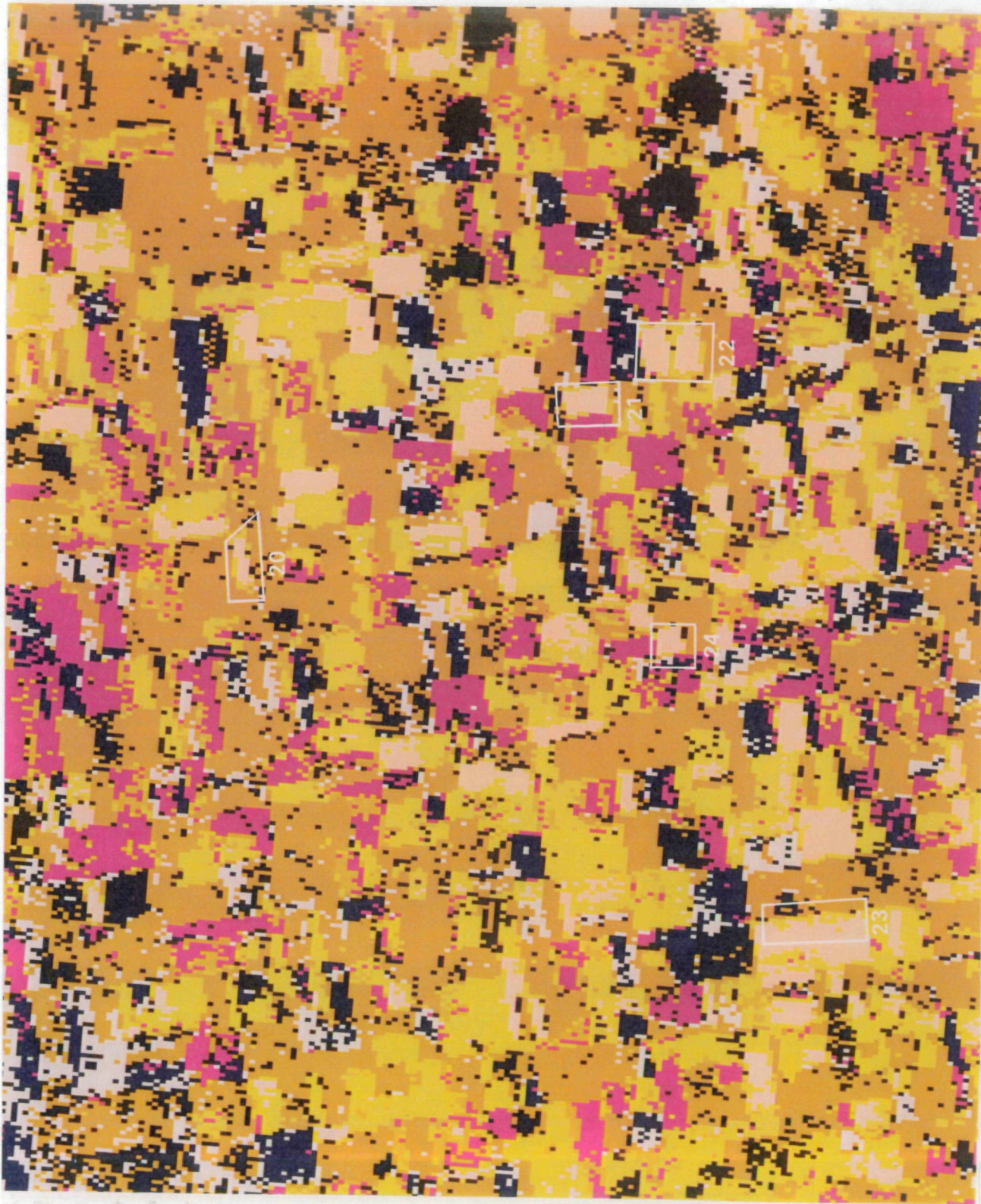
Fig. 3-5 Categorized Imagery - Bendix Restoration Original Sampling Interval, Assumed S/N = 30
