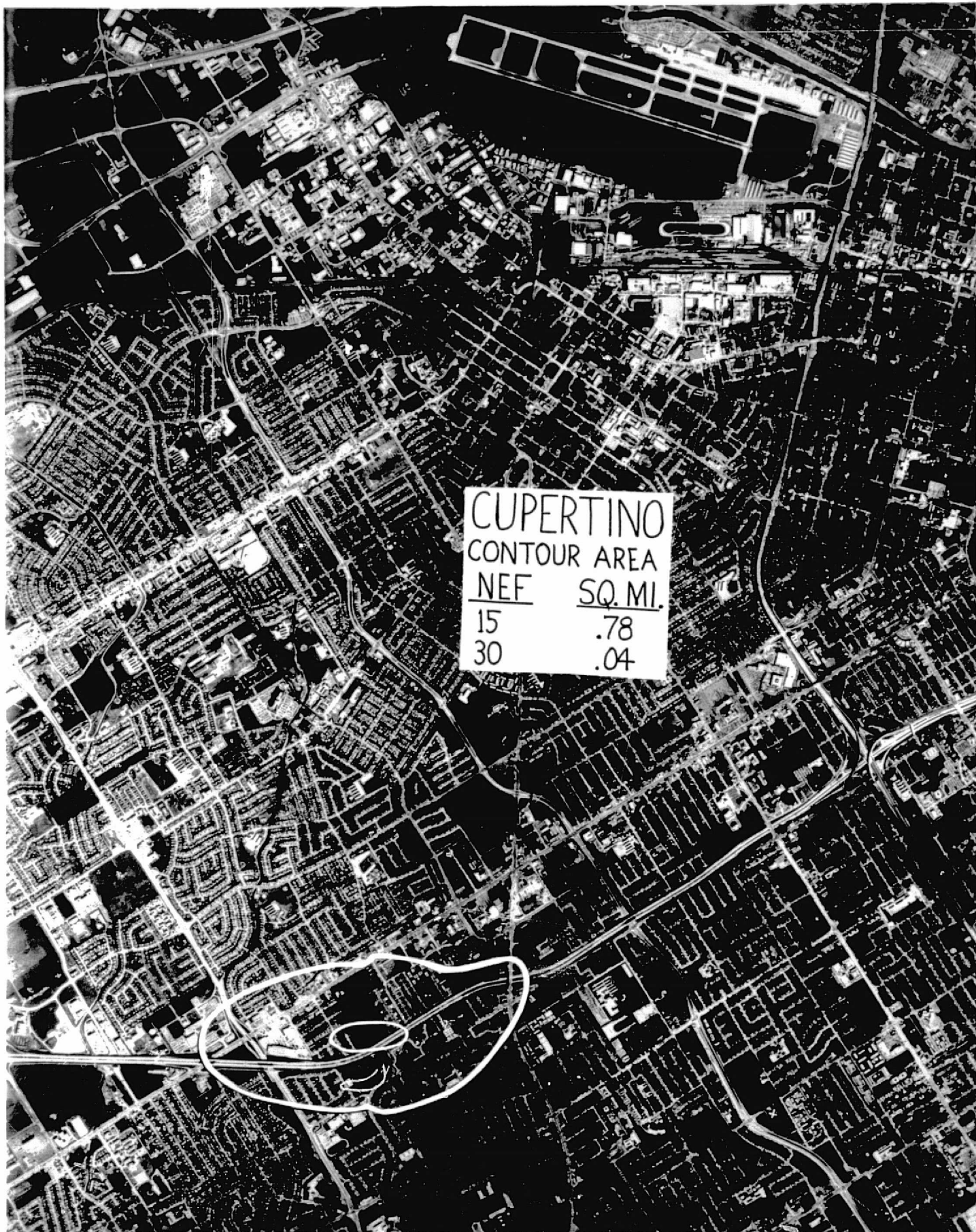
Figure 19. Estimated NEF Contours for Operations of the Conceptual Tilt Rotor Aircraft to and from Cupertino (CUP)
