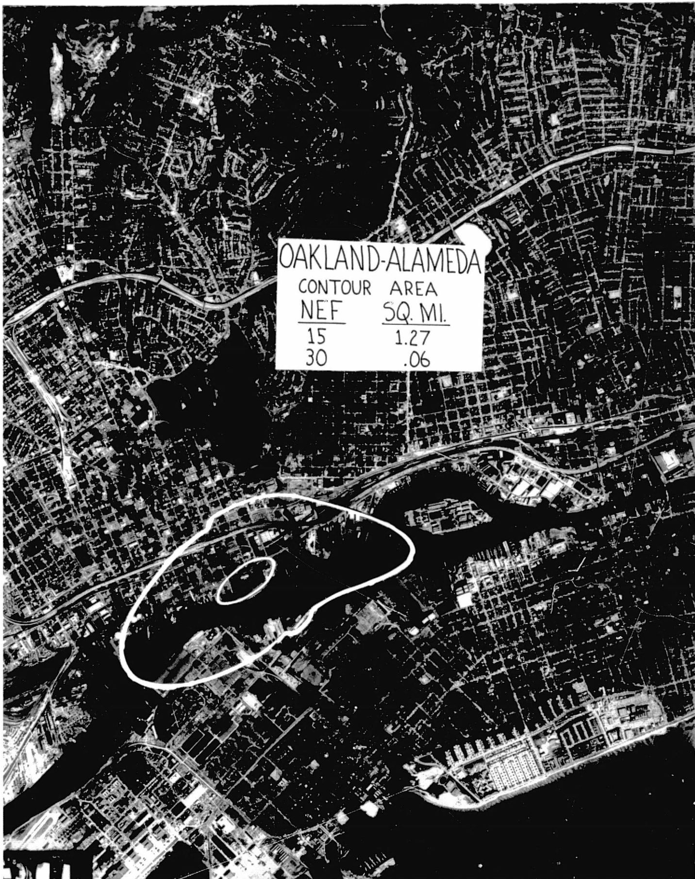
Figure 20. Estimated NEF Contours for Operations of the Conceptual Tilt Rotor Aircraft to and from Oakland (JLS)
