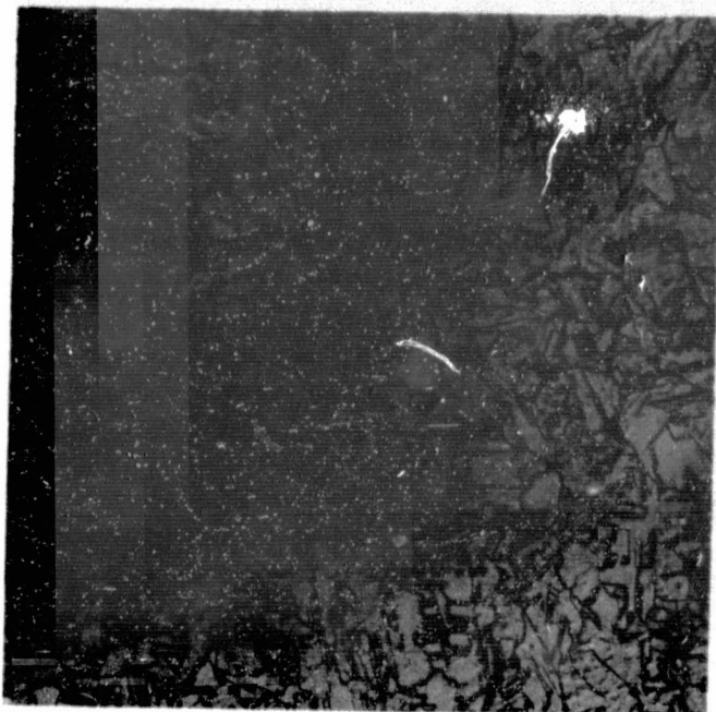
Fig. I-62. Grain characteristics at 0.7-mm from crucible bottom (10X).
