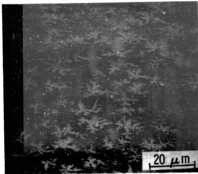
Fig. II-19(a) SEM surface image of silicon carbide dendrites on ribbon surface.
