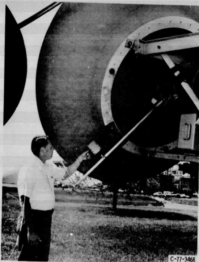
Figure 5. - Rear view of nodding feed antennae.
