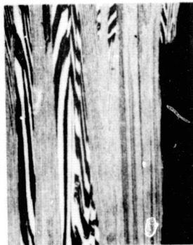
Figure 5. - Shear failures of tensile shear specimens, longitudinal views.
