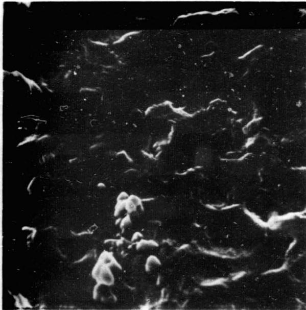
(a) AS RECEIVED, ANNEALED ZIRCALOY-2, 40-kg LOAD, 40 Pa I<sub>2</sub>,
