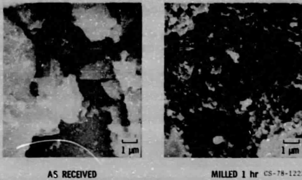
Figure 3. - As received and attrition milled silicon powder; SEM; X10 000.
