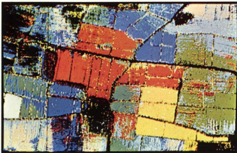
Fig. 24 - Classification results of rice varieties with ML method after data compression from 8 to 5 dimensions, by principal components analysis.
