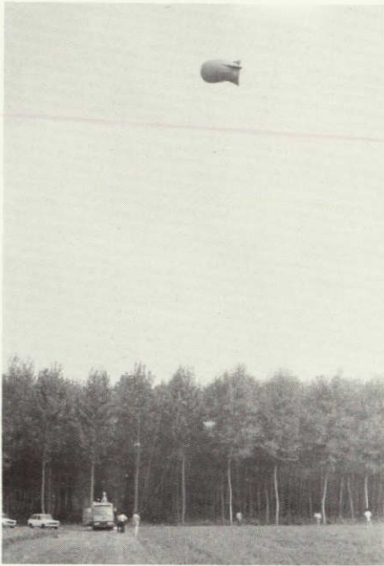
Fig. 118 - Captive balloon for spectral signature measurements above poplar groves
