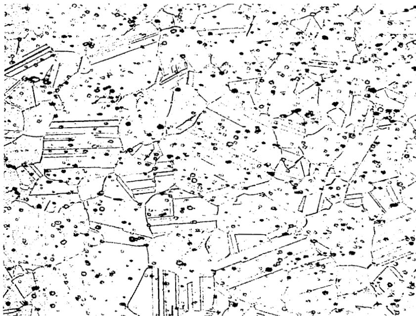
Figure 53: Microstructure of .76 mm (0.030 inch) Thick Supplementary Grain Size Study Sheet Produced from Heat 4-1697. Grain Size ASTM 5-6, Predominantly 5-1/2. X300.
