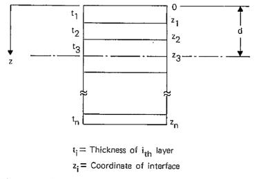
Fig. 1 - Cross Section of n layer Composite Beam
