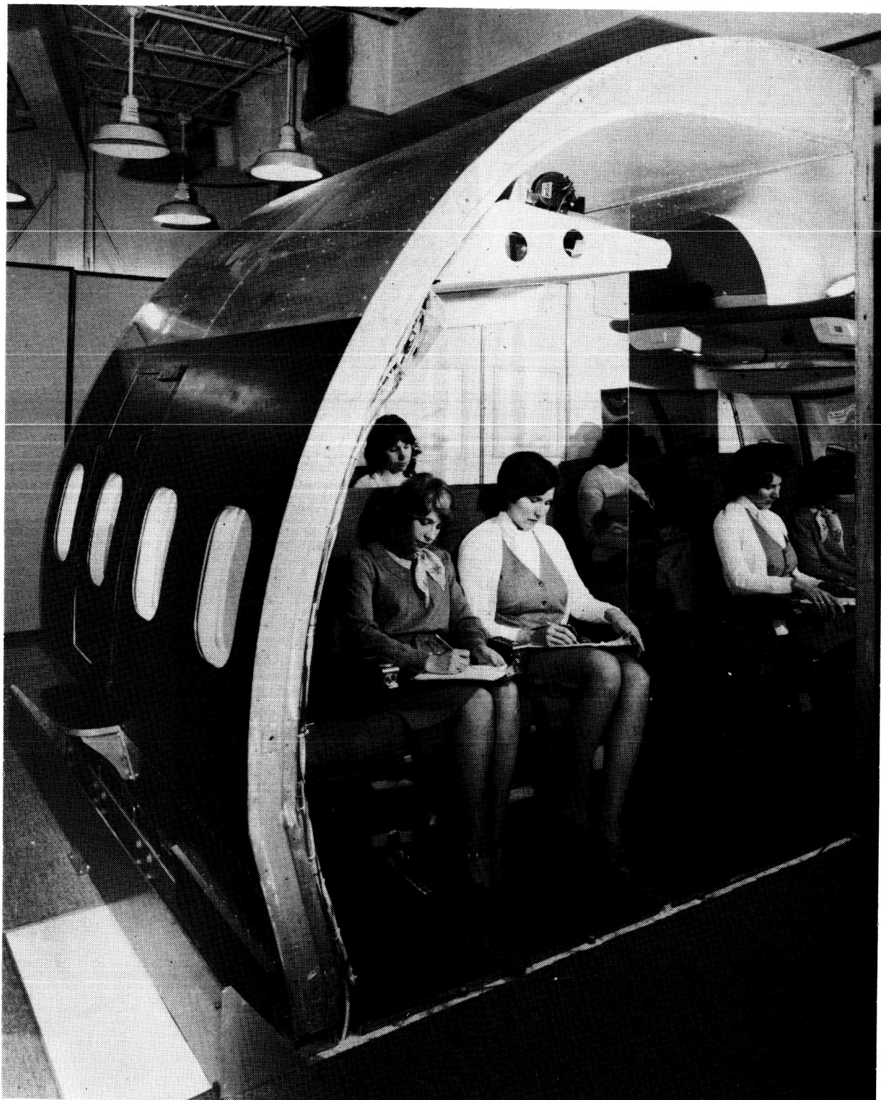
Figure 1.- Langley passenger ride quality apparatus.
